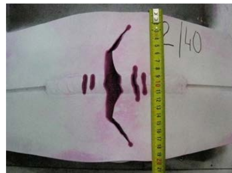
Fig. 8. Indications developed in the penetrant tests and involving the cracks formed after bending the second 40 mm thick specimen
