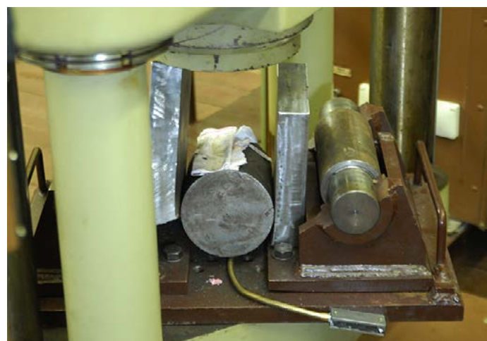
Fig. 9. Fractured specimen sampled from the 60 mm thick material
