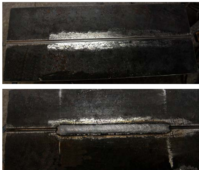
Fig. 3. Specimen before surfacing and with the overlay weld
