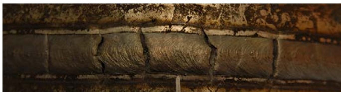
Fig. 5. Initial stage of crack formation induced in the overlay weld of the specimen subjected to bending
