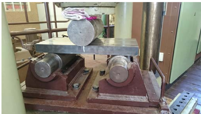
Fig. 4. Specimen in the bending device placed in the testing machine
