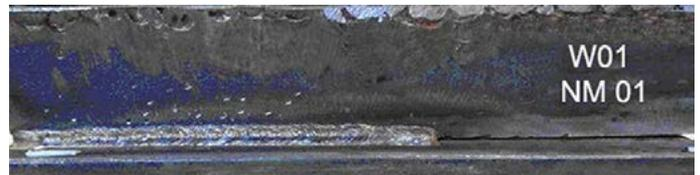
Fig. 1. T-joint with the fillet weld (FW) on the side welded using a non-magnetised electrode
