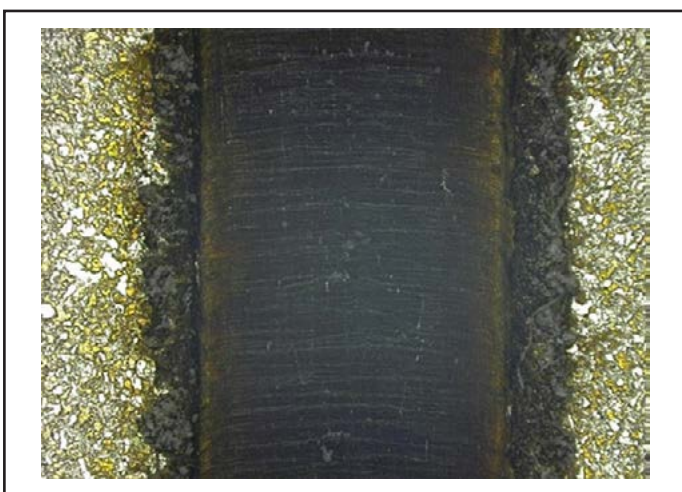
Figure 4. Laser Ablation of AlSi coating for high-strength steel welding. High pulse energy fiber laser technology delivered through a novel square fiber efficiently ablates the AlSi coating to expose the native steel surface for enhanced weld quality.
