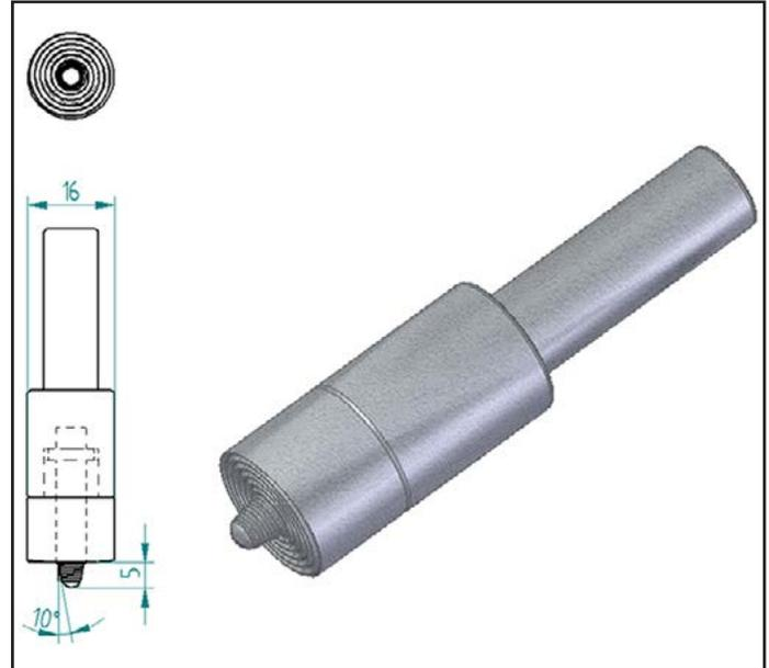
Rys. 5. Shape and dimension of the tool used in the real FSW process
