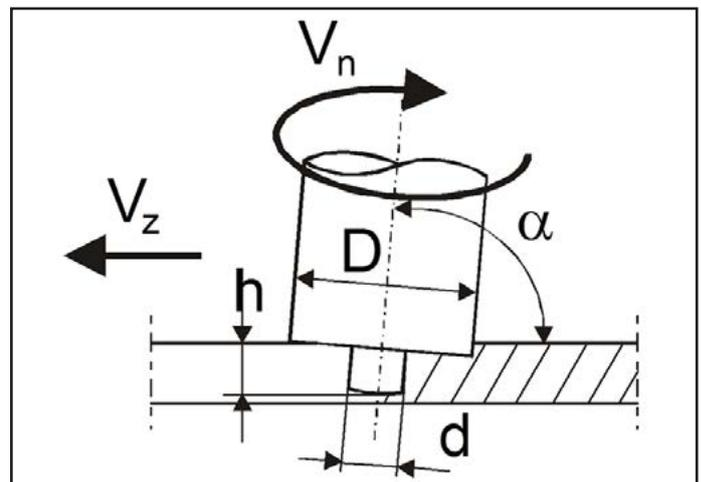
Fig. 1. Scheme of tool movement during FSW ( $v_n$  – rotation rate,  $v_z$  – tool linear velocity) [6]
