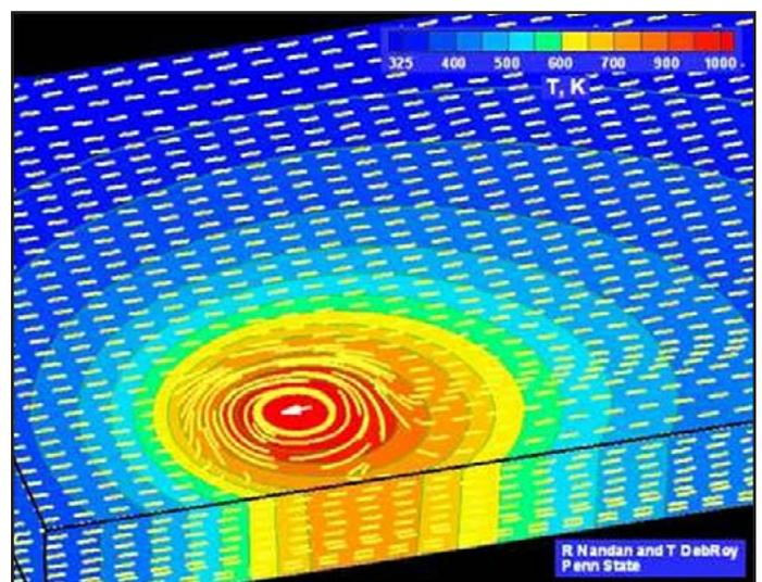
Fig. 2. Results of simulation of FSW welding process – temperature field and directions of the material flow [8]
