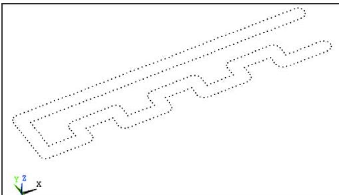
Fig. 8. FSW process path in FEM model
