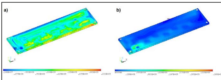
Fig. 13. Values of a) reduced stress (according to the Huber - Mises – Hencky hypothesis) 457 seconds following the welding process start, b) residual stress (5400 seconds following the welding process completion)
