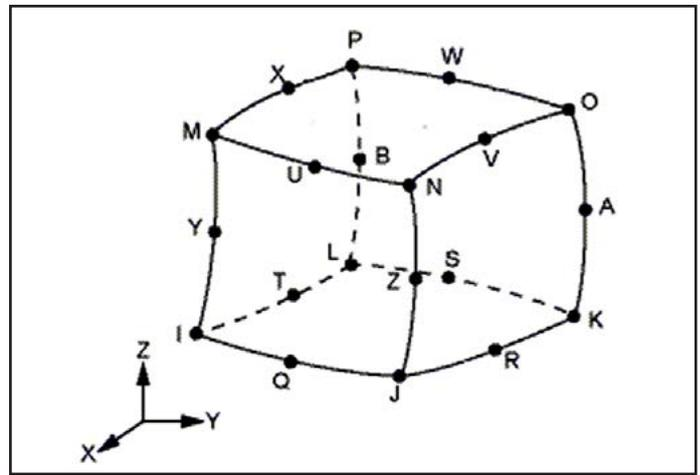
Fig. 9. SOLID226 three-dimensional thermo-mechanical solid element
