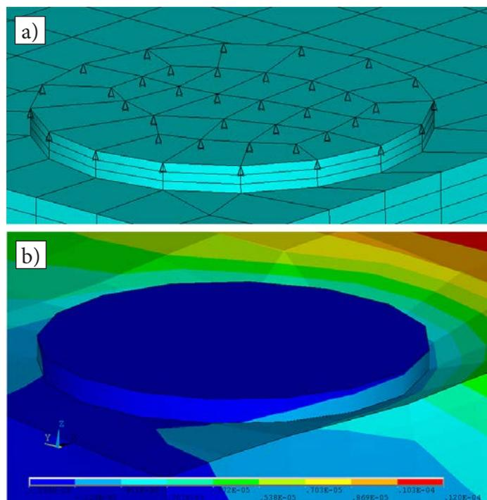
Fig. 11. Nodes of clamps displaced towards axis Z, a) elements, b) value of displacement, mm
