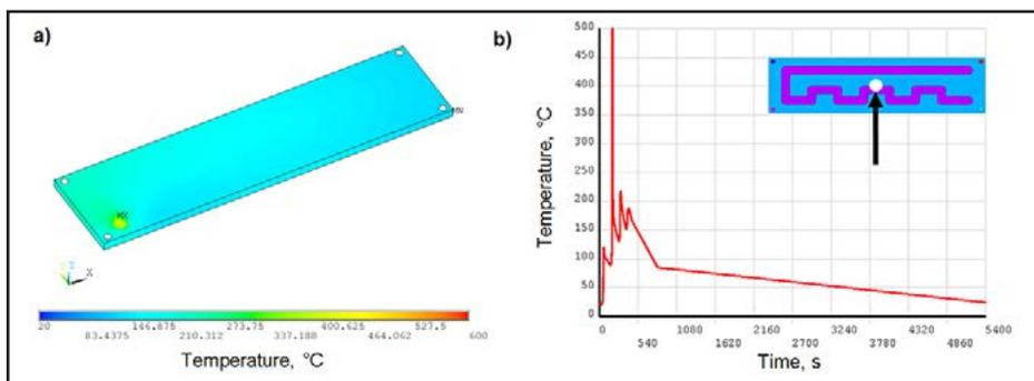
Fig. 12. Temperature analysis a) temperature field after 457 seconds following the welding process start, b) temperature changes in the function of time at point indicated by the arrow
