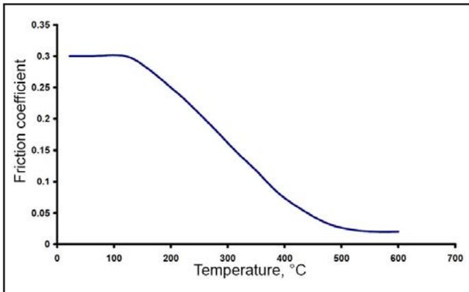
Fig. 3. Dependence of the friction coefficient on the 6061-T6 aluminium alloy temperature [7]
