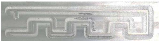
Fig. 4. Model Heat exchanger for tooling testing
