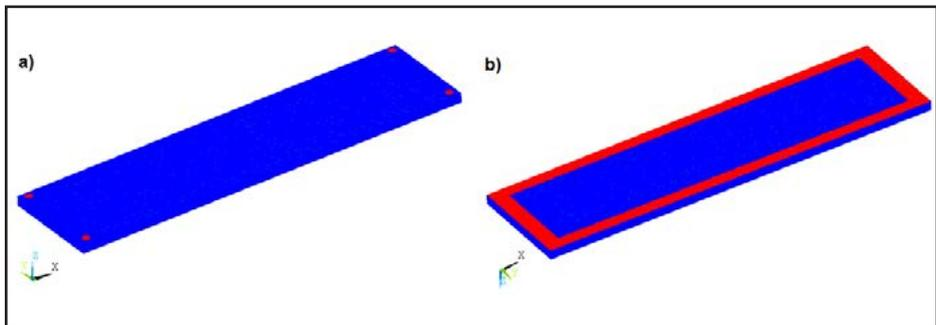
Fig. 10. Reactions of clamps on elements being welded (marked red) a) top view - clamps, b) bottom view - pads
