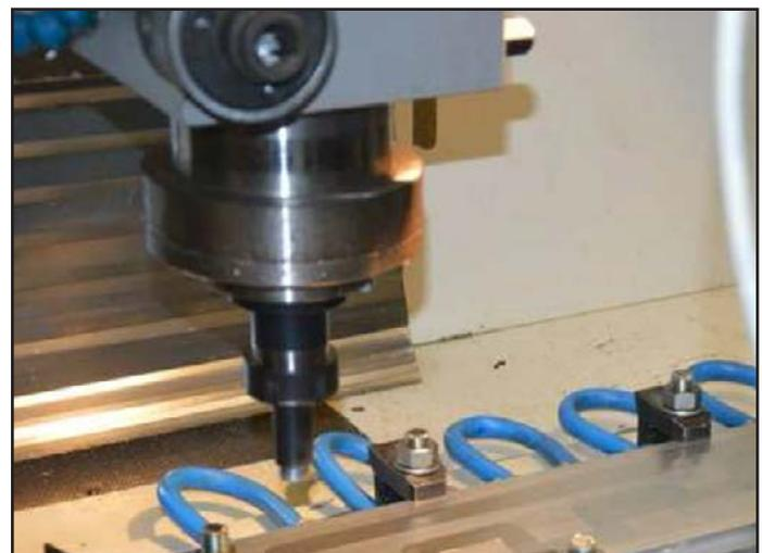
Fig. 6. Station for FSW of the components of the heat exchanger
