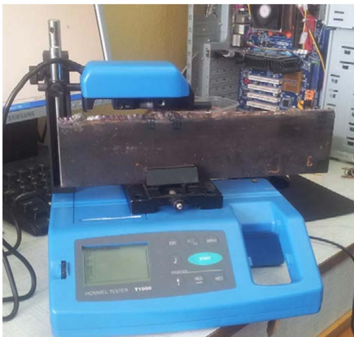
Fig. 11. Hommel tester T1000 contact profile measurement gauge
