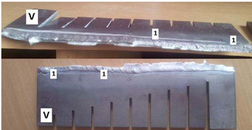
Fig. 10. Butt joint made of aluminium alloy after breaking in the crack formation area. Roman digits represent numbers of successive joints; Arab digits represent number of successive cracks in a given joint
