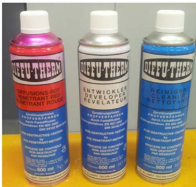
Fig. 7. Set of aerosols “Diffu - Therm” used in the penetrant tests of the cracks
