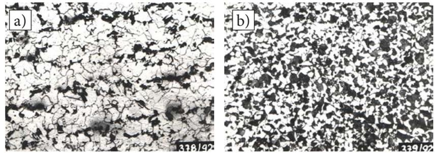
Fig. 4. Structure of the overlay weld ( $g=1$  mm) and the heat affected zone (HAZ) of the specimen surfaced using process 111 and subjected to normalising: a) overlay weld structure – ferrite + pearlite, etchant: Nital; 250x magnified; b) HAZ structure – pearlite + ferrite, etchant: Nital; 250x magnified
