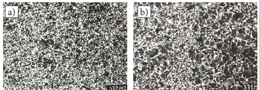
Fig. 5. Structure of the overlay weld ( $g=1$  mm) and of the HAZ of the specimen surfaced using process 111 and subjected to toughening: a) structure of the overlay weld – pearlite + ferrite, etchant: Nital; 250x magnified; b) structure of the HAZ – pearlite + ferrite, etchant: Nital; 250x magnified
