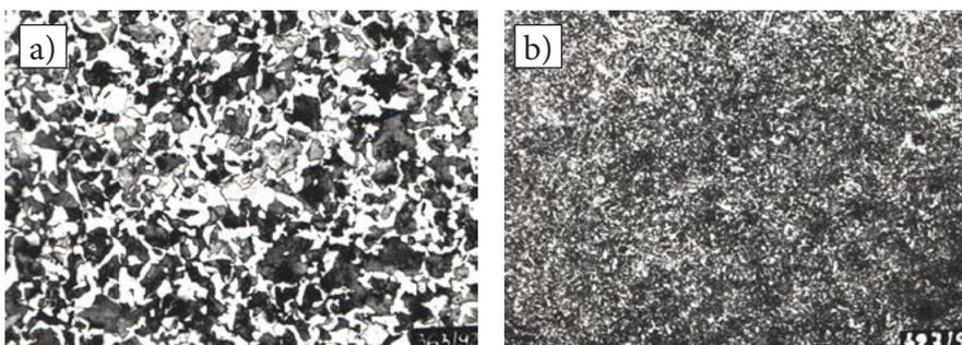
Fig. 3. Structure of steel C45: a) after normalising – pearlite + ferrite; etchant: Nital; 250x magnified; b) after toughening – highly toughened martensite (sorbite), etchant: Nital; 250x magnified;
