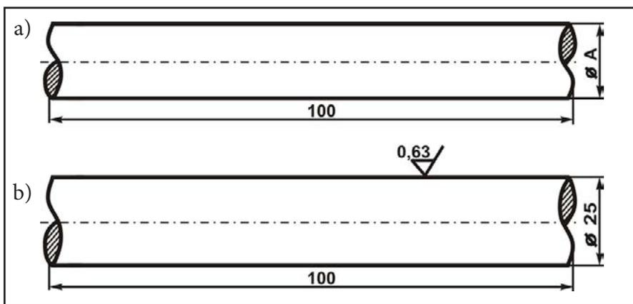
Fig.1. Shapes and dimensions of the test specimens: a) prepared for surfacing:  $A=23$  mm – for the specimens with the surfaced layer having the thickness of  $g=1$  mm,  $A=21$  mm – for the specimens with the surfaced layer having the thickness of  $g=2$  mm; b) after surfacing and mechanical treatment
