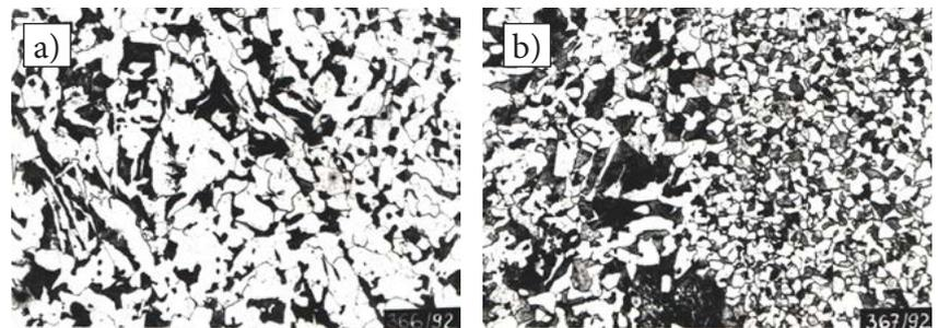
Fig. 6. Structure of the overlay weld ( $g=2$  mm) and of the HAZ of the specimen surfaced using process 135 and subjected to normalising: a) structure of the overlay weld – ferrite + pearlite, etchant: Nital; 250x magnified; b) structure of the HAZ – ferrite + pearlite, etchant: Nital; 250x magnified
