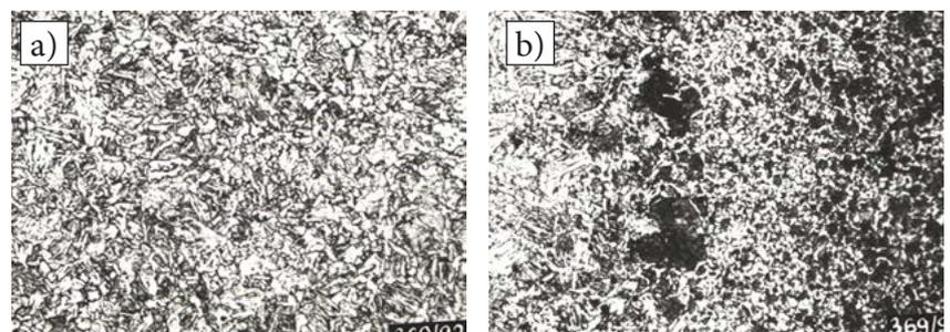
Fig. 7. Structure of the overlay weld ( $g=2$  mm) and of the HAZ of the specimen surfaced using process 135 and subjected to toughening: a) structure of the overlay weld – ferrite + pseudo pearlite + traces of bainite, etchant: Nital; 250x magnified b) structure of the HAZ – ferrite + pseudo pearlite + traces of bainite, etchant: Nital; 250x magnified
