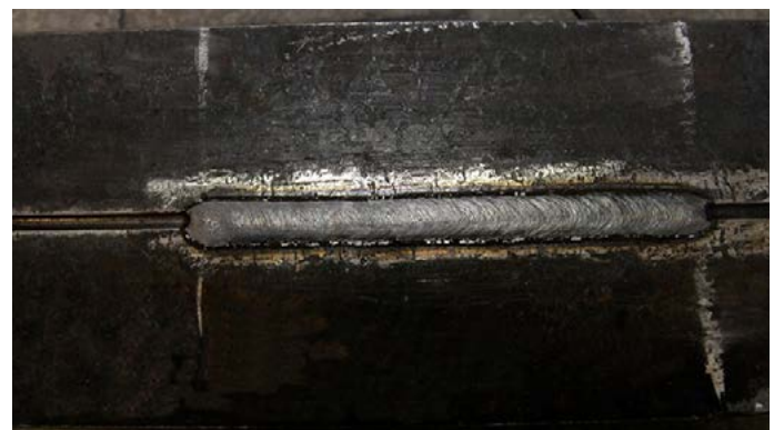
Fig. 6. Test specimen with the overlay weld
