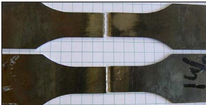
Fig. 9. Photographs of the exemplary laser-beam welded specimen after the tensile strength test – rupture in the weld
