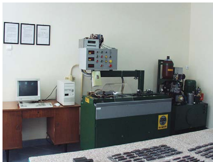
Fig. 4. Main view of the simulator of thermal-strain cycles produced by Instituto Spawalnictwa (version from 1996)
