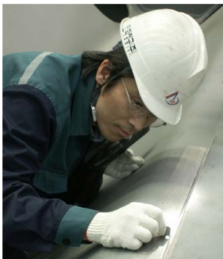
Fig. 8. Depth inspection using simple gauges. The gap between the base plate and the gauge in the right-hand picture indicates that 0.2 mm has not been achieved
