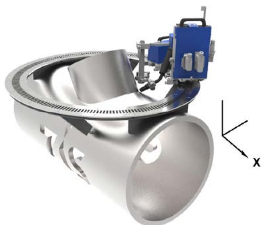
Fig. 12. CAD model of a system on a rail for welding tube and socket connections
