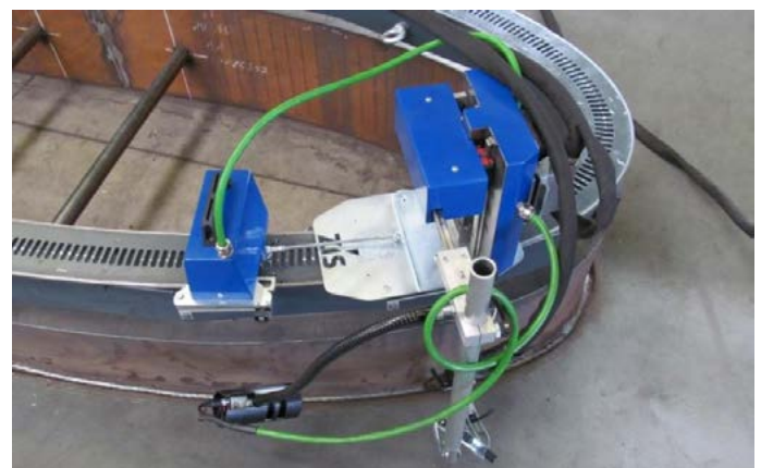
Fig. 11. System on rails for welding in door frames
