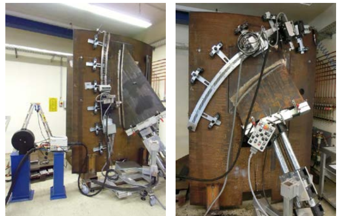
Fig. 6. Tube segment clamped in positions PF and PFO45
