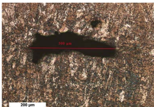
Fig. 10. Size of the gas pore in joint no. 3
