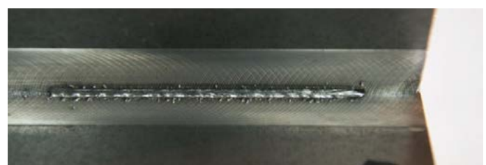
Fig. 7. Double-sided T-joint with a proper weld face
