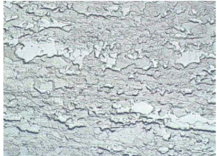
Fig. 1. Bainitic-ferritic structure of steel S700MC
