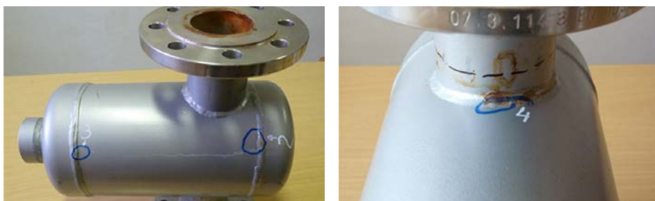
Fig. 7 Leakages in weld of air separator unit
