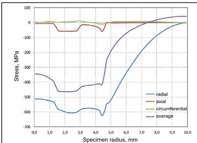
Fig. 15. Distributions of stress constituents (radial, axial and circumferential) and of mean stress along the radius of the AlN specimen
