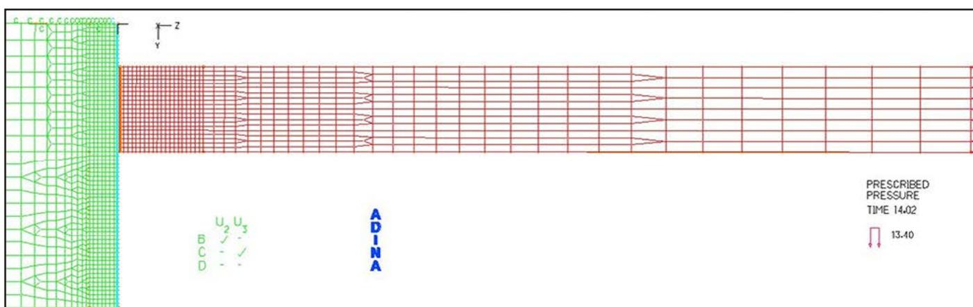
Fig. 3. FEM mesh of the AlN-Ti mechanical model with designated boundary conditions
