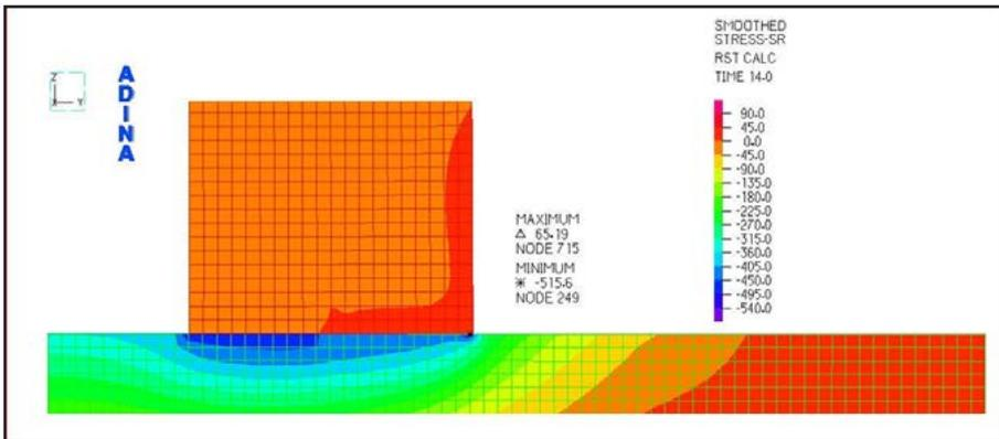
Fig.12. Distribution of mean stresses  $\sigma_{sr}$  near the interface surface at the final stage of friction-induced heating
