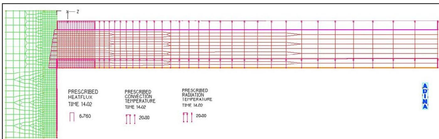
Fig. 2. FEM mesh of the AlN-Ti thermal model with boundary conditions
