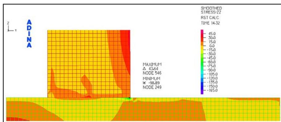
Fig. 9. Distribution of axial stresses  $\sigma_{zz}$  near the interface surface after releasing the load and heat stream from friction (0.32 s)
