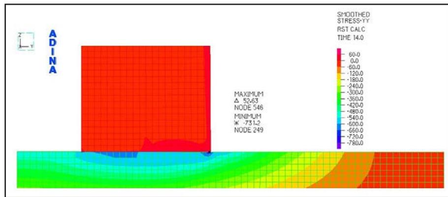
Fig. 6. Distribution of radial stresses  $\sigma_{yy}$  near the interface surface at the final stage of friction-induced heating
