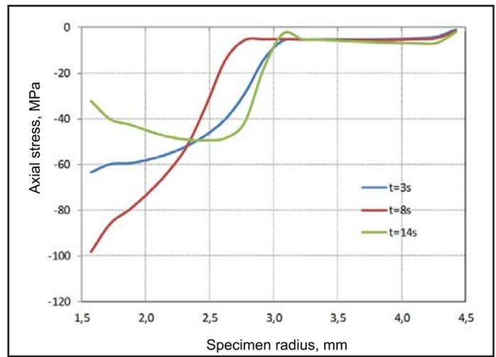
Fig. 14. Radial distributions of axial stresses in the joint: a) on the AlN ceramics side, b) on the titanium side
