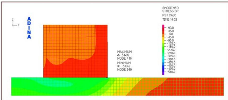
Fig. 13. Distribution of mean stresses  $\sigma_{sr}$  near the interface surface after releasing the load and heat stream from friction (0.32 s)
