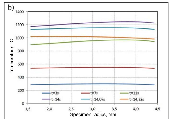
Fig. 5. Radial distributions of temperature on the AlN-Ti joint boundary: a) on the AlN ceramics side, b) on the titanium side
