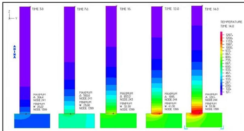
Fig. 4. Maps of temperature distribution for selected times of the friction-induced heating of the AlN ceramics with titanium
