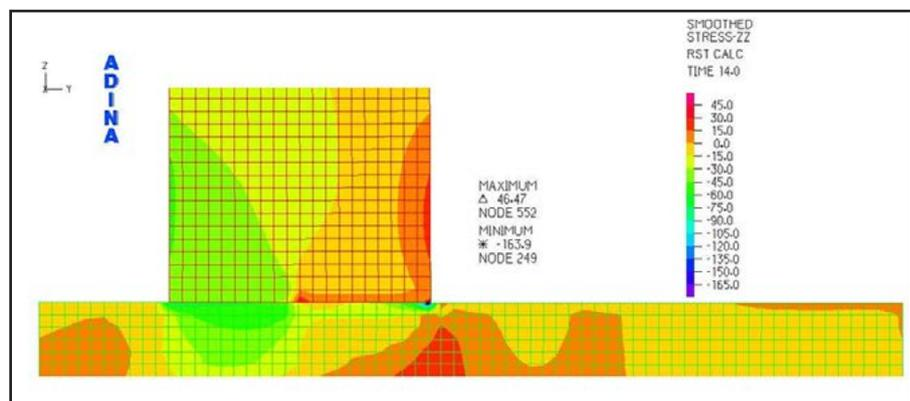
Fig. 8. Distribution of axial stresses  $\sigma_{zz}$  near the interface surface at the final stage of friction-induced heating
