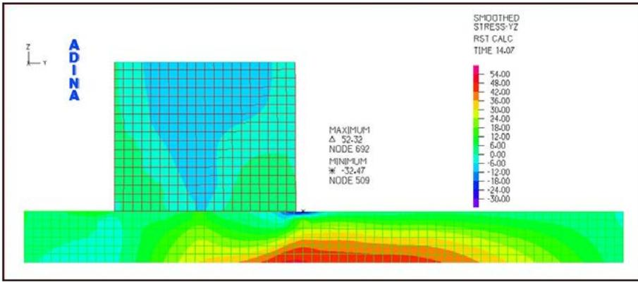
Fig.10. Distribution of circumferential stresses  $\sigma_{yz}$  near the interface surface at the final stage of friction-induced heating
