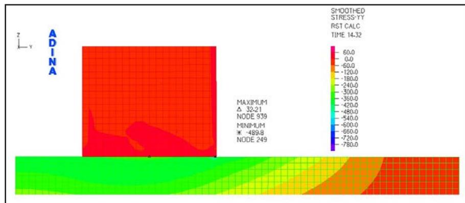
Fig. 7. Distribution of radial stresses  $\sigma_{yy}$  near the interface surface after releasing the load and heat stream from friction (0.32 s)
