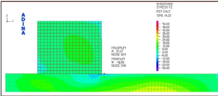
Fig. 11. Distribution of circumferential stresses  $\sigma_{yz}$  near the interface surface after releasing the load and heat stream from friction (0.32 s)
