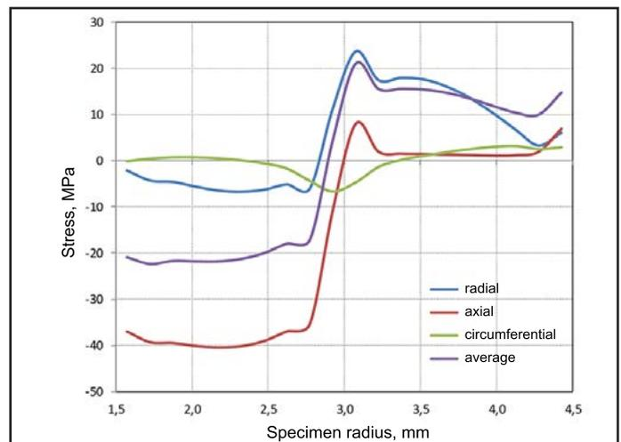
Fig. 16. Distributions of stress constituents (radial, axial and circumferential) and of mean stress along the radius of the titanium specimen
