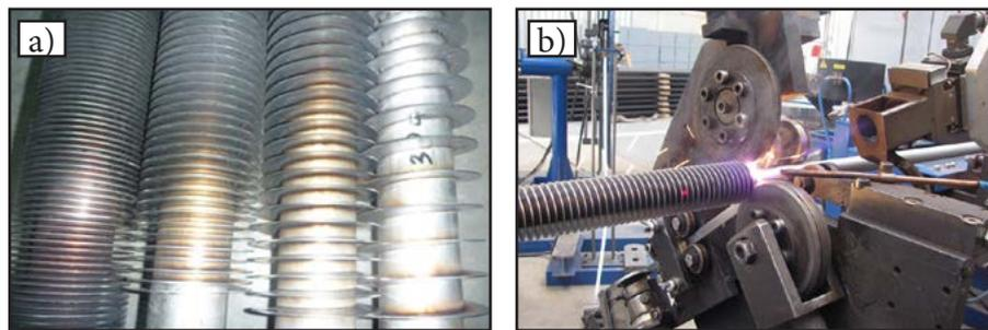
Fig. 3. Fin tubes made of alloy Inconel 625 at Energoinstal SA (a), laser welding of tubes (b) [2]
