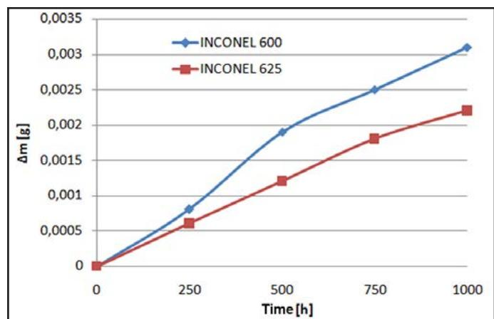
Fig. 10. Change in the weight of laser welded fin tube specimens (with the weld under the fin) made of Inconel 600 and Inconel 625
