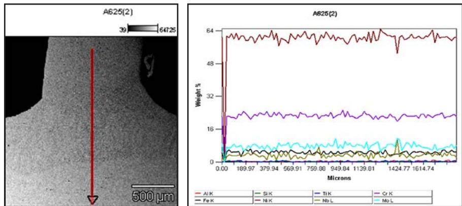
Fig. 5. Results of the chemical composition microanalysis (EDS) involving the cross-section of the joint – linear distribution
