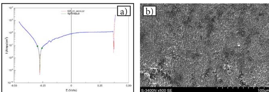
Fig. 12. Polarisation curve with the Stern-Geary adjustment in the cathodic-anodic range related to the weld specimen made of alloy Inconel 625 (a), surface structure after tests concerning resistance electrochemical corrosion in the 3.5% NaCl solution (b)
