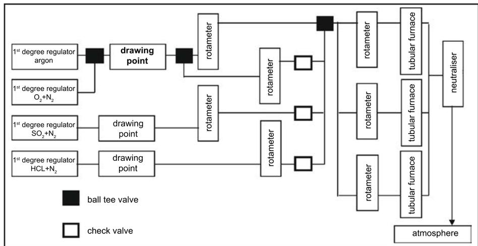
Fig. 9. Scheme of the test rig for investigating high-temperature corrosion of fin tubes
