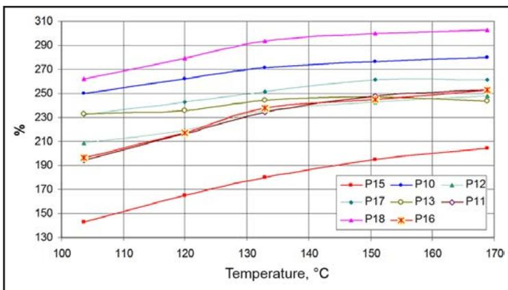
Fig. 8. Relative heat flux emitted by steam through test tubes to air compared to heat flux emitted through smooth tube
