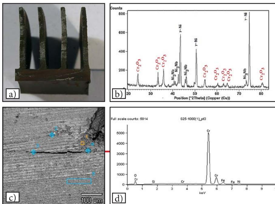
Fig. 11. Test results related to the laser-welded tube-fin joint made of alloy Inconel 625 after the assessment of resistance to high-temperature corrosion in the atmosphere of flue gas for 1000 hours at a temperature of 800°C: a) specimen surface, b) XRD-based phase analysis results of corrosion products, c) EDS-based microanalysis results related to the chemical composition on the specimen surface
