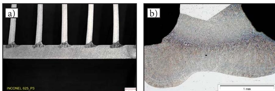
Fig. 4. Structure of the laser-welded fin tube made of alloy Inconel 625: a) macrostructure b) microstructure of the tube-fin joint
