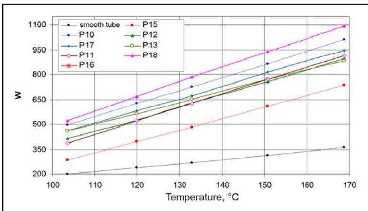
Fig. 7. Measured heat flux emitted by steam through test tubes to air
