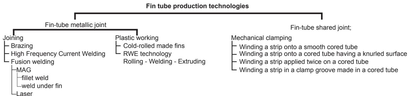
Fig. 1. Division of fin tube production technologies [4]
