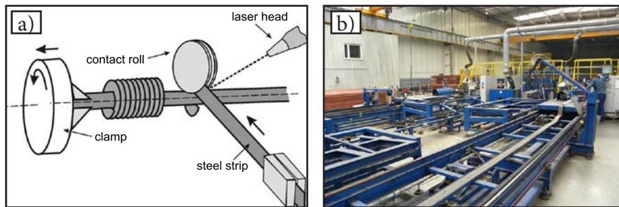
Fig. 2. Laser welding of fin tubes: a) schematic diagram of the welding station, b) automated line for the welding of fin tubes at the Centre for Innovative Laser Technologies (CITL) Energoinstal SA [5]
