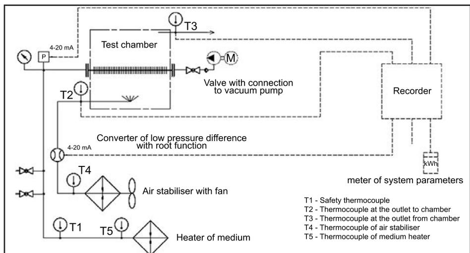
Fig. 6. Schematic diagram of the test rig for measuring the thermal efficiency of fin tubes
