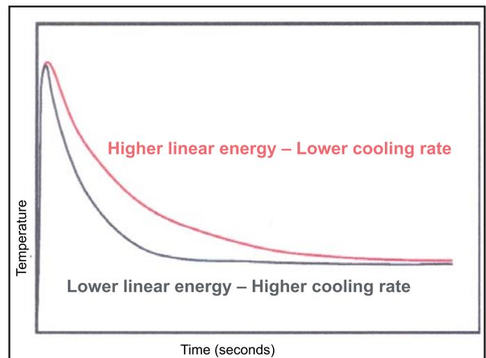
Fig. 1. Effect of welding linear energy on welding rates [1]
