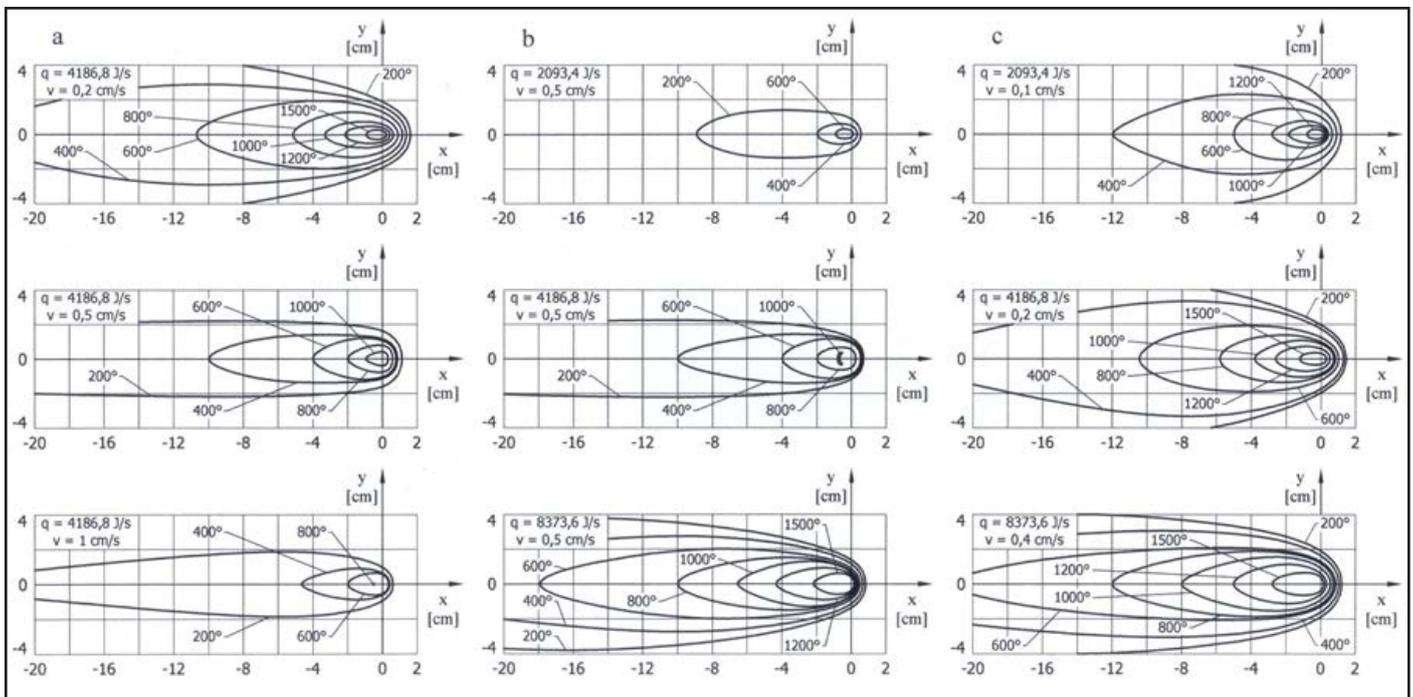
Fig. 2. Nearly stabilised thermal field in relation to various welding parameters [11]
