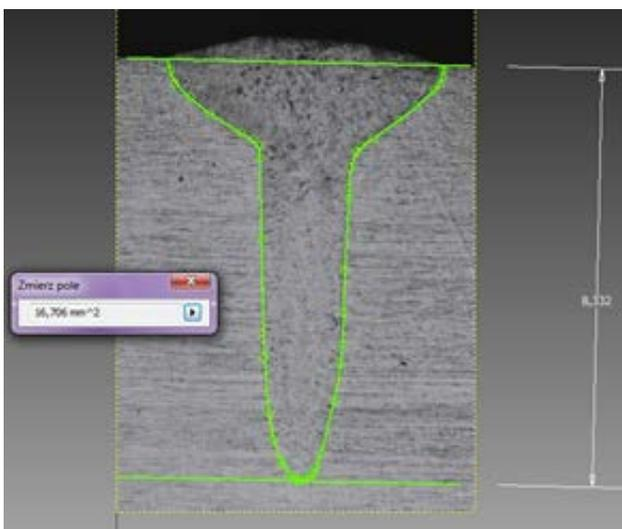
Fig. 4. Planimetric measurement of the area of the butt weld made using electron beam welding; the measurement was performed using the Autodesk Inventor Professional software programme – student’s version
