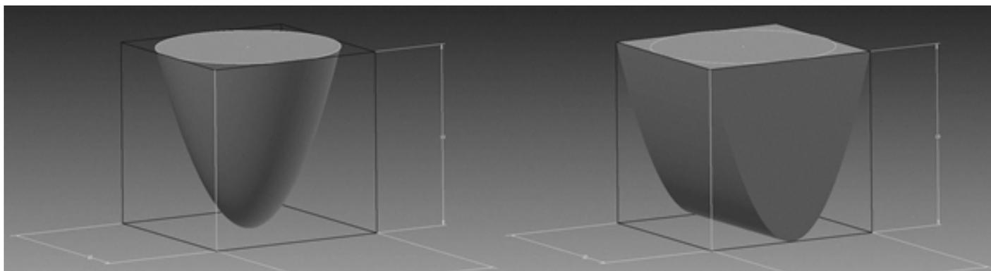
Fig. 6. Manner of assessing the heat input during spot welding
