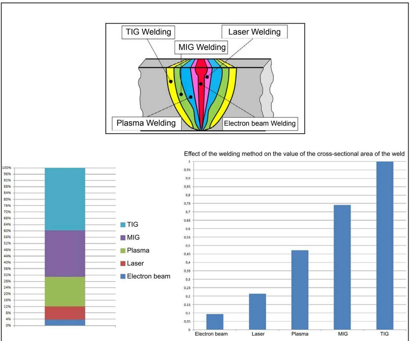
Fig. 3. Comparison of heat input supplied during TIG, MIG, plasma, laser and electron beam welding [14]
