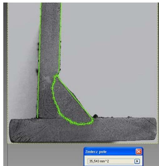
Fig. 5. Planimetric measurement of the area of the fillet weld made using the MAG method; the measurement was performed using the Autodesk Inventor Professional software programme – student’s version
