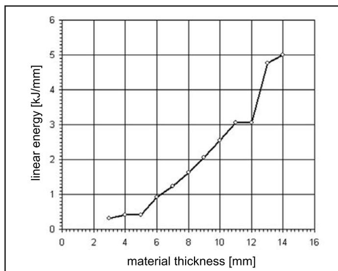
Fig. 7. Change in linear energy when welding unalloyed and low-alloy structural steels, a – standardising through the measurement of cross-sectional areas, b – standardising through the estimation of external parameters [15]
