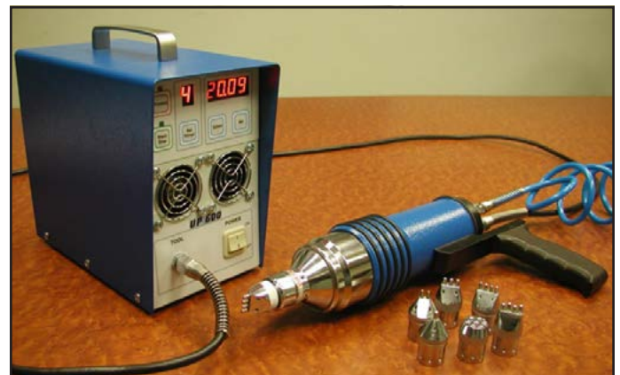
Fig. 3. Basic ultrasonic peening system for treatment of welded elements and structures [7]
