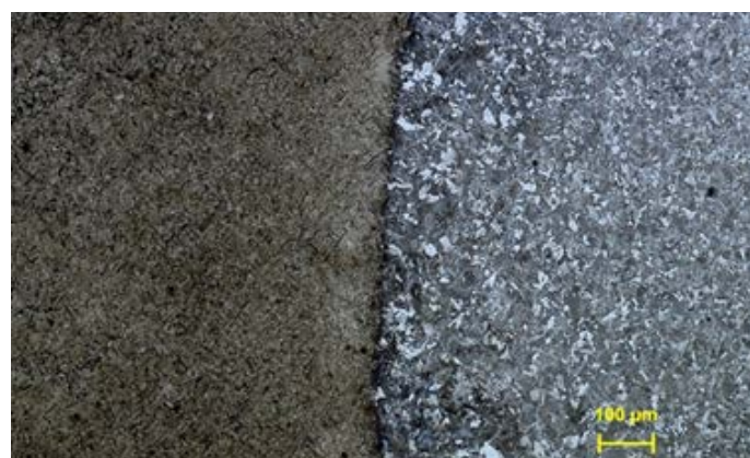
Fig. 12. Microstructure of the joint-pipe welding line
