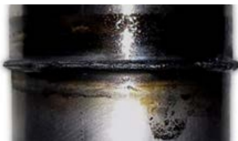
Fig. 8. Effect of the welding of oiled butting faces of elements
