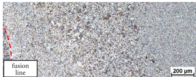
Fig. 5. Location of HAZ zones, the second repair joint; TIG welding method; weld on the left
