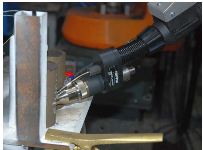
Fig. 2. Welding station used for the performance of TOP-TIG™ method-based repair welding
