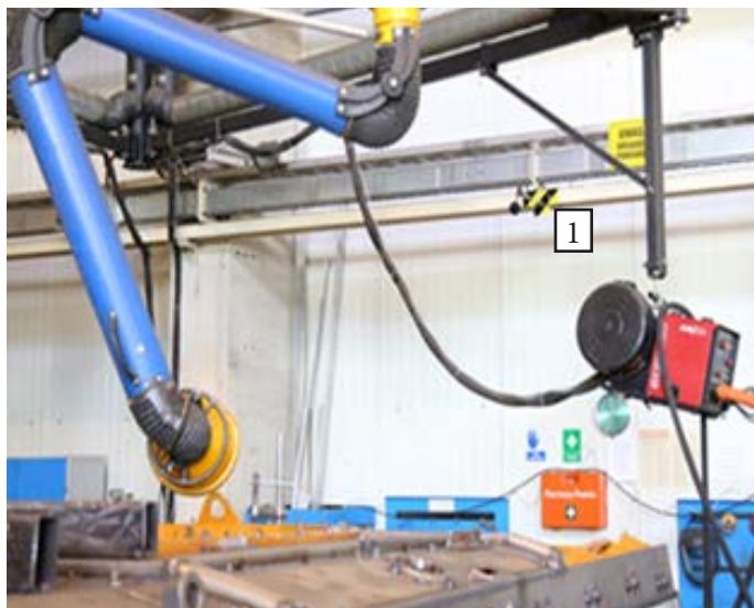
Fig. 4. System measurement microphones located at various production areas; 1 – microphone
