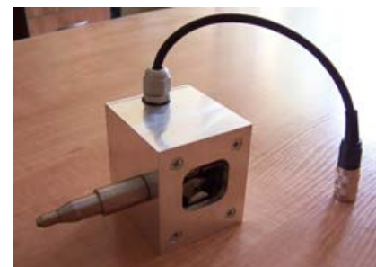
c) transducer for measurements of filler metal wire feeding rates installed in the filler metal wire feeder
