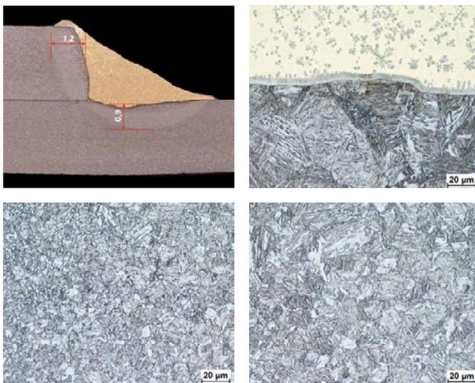
Fig. 2. Macro and microstructure of the MAG arc braze welded joint made using a linear energy of 0.17 kJ/mm: joint macrostructure (a), brazeweld microstructure (b), HAZs (c and d)
