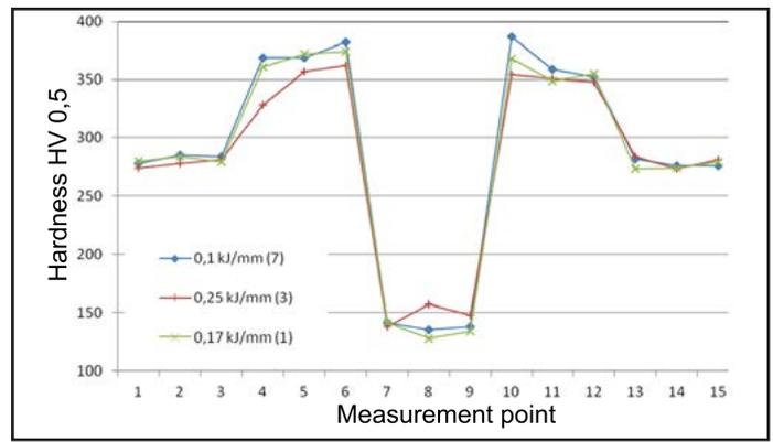
Fig. 3. Arrangement of measurement points on the cross-sections of braze welded joints (a) and hardness distribution on the cross-sections of braze welded joints made using the MAG method and a linear energy of 0.1 kJ/mm – specimen no. 7, 0.25 kJ/mm – specimen no. 3, 0.17 kJ/mm – specimen no. 1
