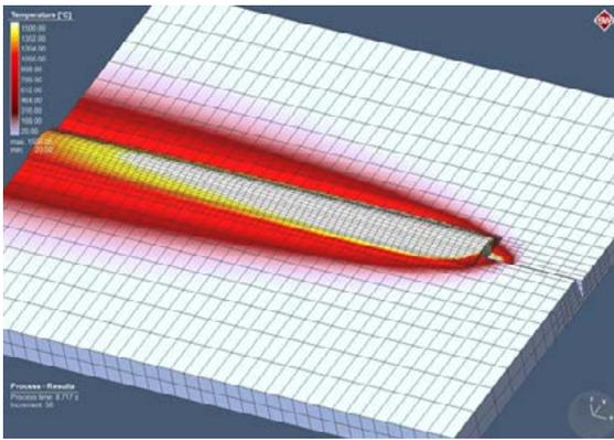
Fig. 3. Simulation of the hybrid welding of stainless steel S960QL joint using the simufact.welding software programme and the condensation of the finite element mesh within the heat source
