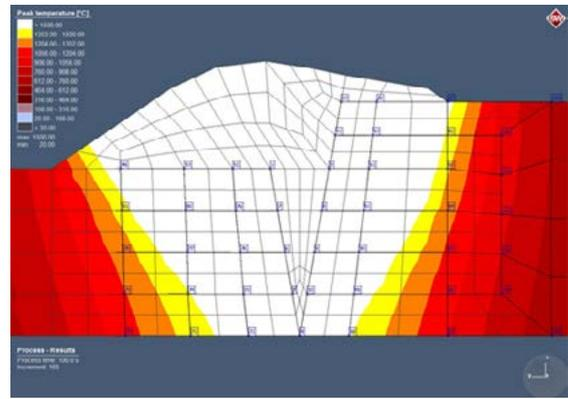
Fig. 4. Distribution of maximum temperatures in the welded joint and the measurement points for which the temperature values were recorded in the function of time
