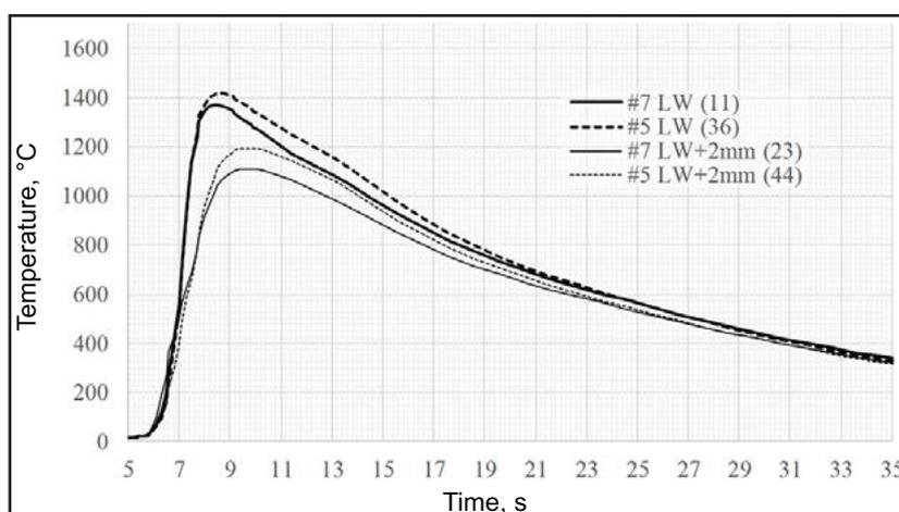
Fig. 7. Temperature changes in the HAZ; #7/#5 - sheet thickness; mm; L - weld face area, LW - fusion line area
