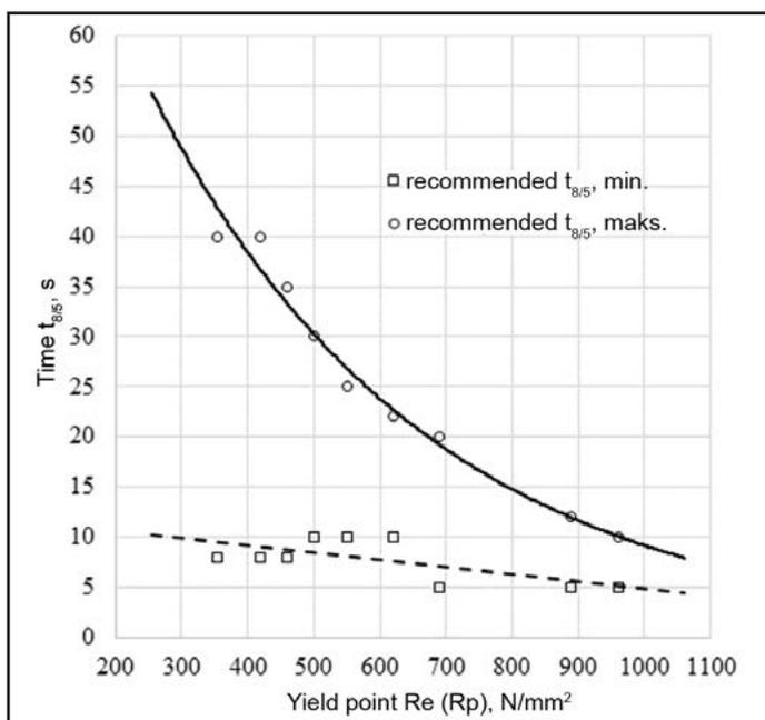
Fig. 1. Recommended times  $t_{8/5}$  for fine-grained structural steels [6]
