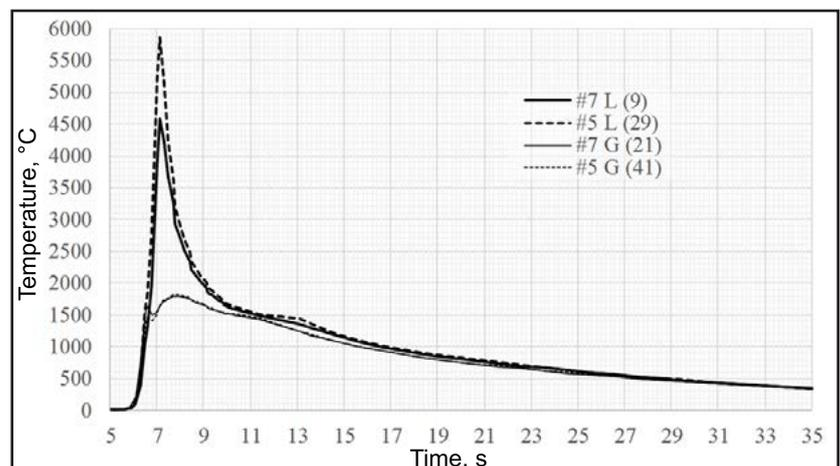
Fig. 5. Temperature changes in the weld axis #7/#5 - sheet thickness, mm; L - weld face area, G - weld root area
