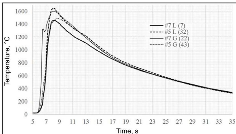
Fig. 6. Temperature changes in the weld at the fusion line; #7/#5 - sheet thickness; mm; L - weld face area, G - weld root area
