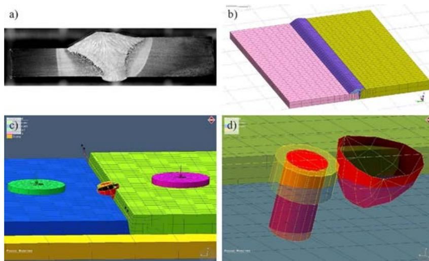
Fig. 2. Geometry of the joint and method of the modelling the hybrid heat source: a) macroscopic image of the welded joint of 5.0 mm and 7.0 mm thick sheets b) space model of the joint – the finite element mesh in the midas NFX software programme; c) definition of the welding process in the simufact.welding software programme allowing for support, the pressure of each of the welded plates and the appropriate trajectory for the heat source; d) geometry of the hybrid heat source
