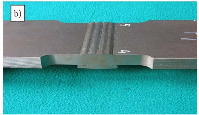
Fig. 2. Shape and dimensions of the specimens subjected to fatigue tests: a) schemes of the specimens, b) view of the specimen
