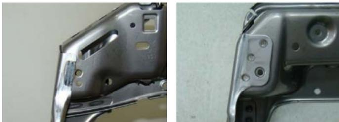
Fig.1. Comparison of the design of the overlap in laser weld and spot-weld
