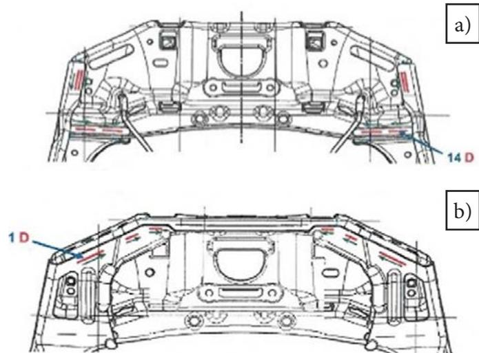
Fig. 2. Location of test welds: a) front view, b) rear view
