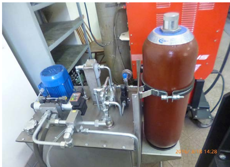
Fig. 4. Supply system of the SHZ 084/14 hydraulic actuator
