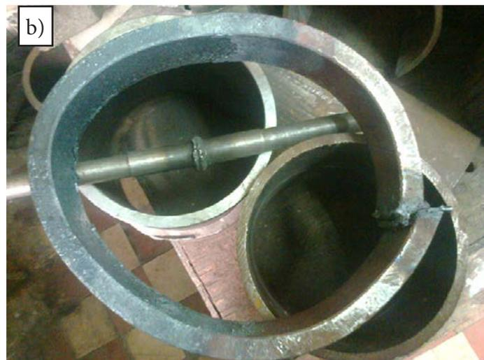
Fig. 6. Butt welding of the ring-shaped product: a) element in the K724 welding machine fixing jaws; b) loss of the ring shape by the product
