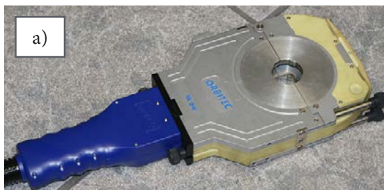
Fig. 1. Heads for orbital TIG welding: a) closed head; b) open head
