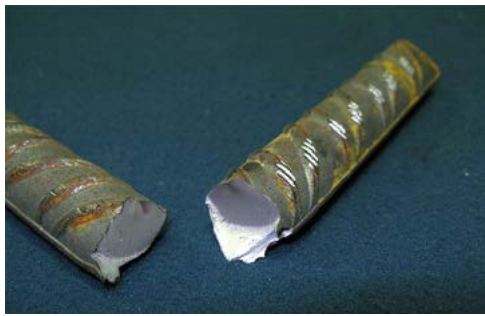
Fig. 7. Cracked bar having a diameter of 20 mm and the fatigue fractures of the bar
