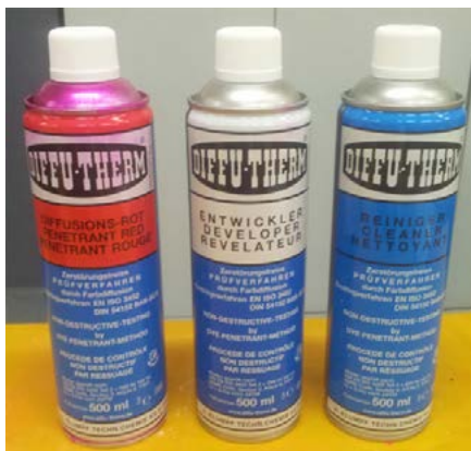
Fig. 3. Set of aerosols "Diffu - Therm" used in the penetrant tests of plates with simulated pores
