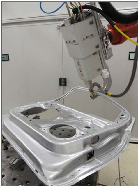
Fig. 5. Welding of 6mm flanges at door frame.
