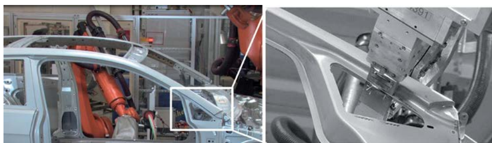
Fig. 2. Car body of Volkswagen Golf VII. Triangle window is welded with LaserSeamStepper.
