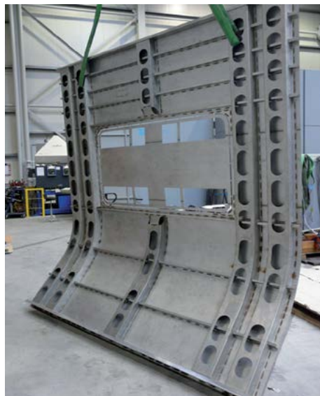
Fig. 10. LaserSeamStepper (picker) welded side panel of a passenger train
