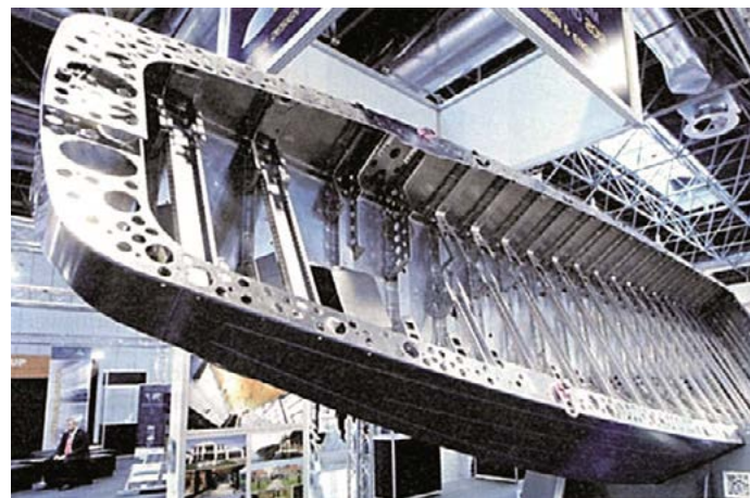
Fig. 8. Aluminum boat hull, welded with LaserSeamStepper in picker version
