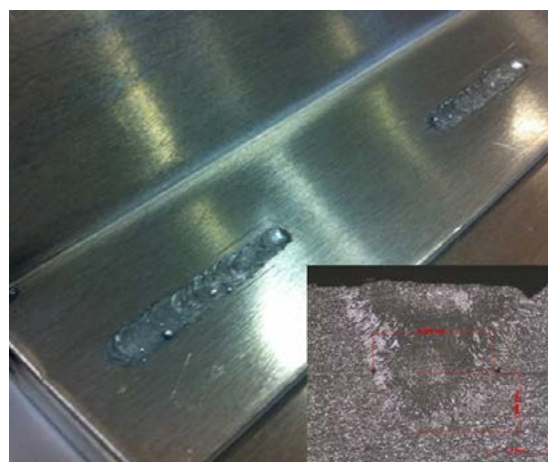
Fig. 9. Large width aluminium weld by oscillated laser beam with LaserSeamStepper in Picker version. Top view (left) and cross section (right)
