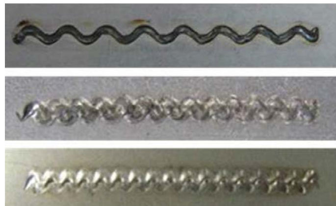
Fig. 1: 40mm weaved seam; upper: MnB-steel, middle: aluminum, lower: stainless steel
