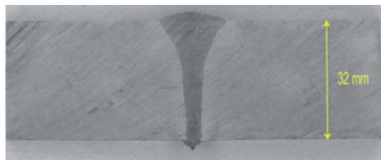
Fig. 13. Type I butt joint made of 32 mm thick alloy steel ( t=32 mm) ; laser power of 30 kW; even thick elements can be welded successfully
