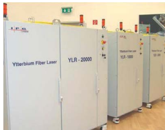
Fig. 5. Fibre laser of many kilowatt power used for welding and cutting thick elements made of alloy steels
