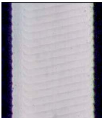
Fig. 3. Trace after removing a layer in the near-edge zone of a thin-layer photovoltaic cell plate
