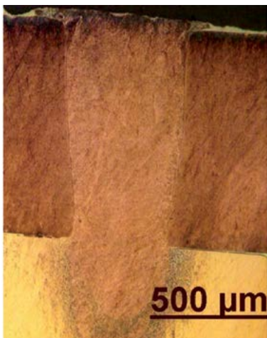
Fig. 7. Metallographic specimen of an overlap joint of a copper contact pin
