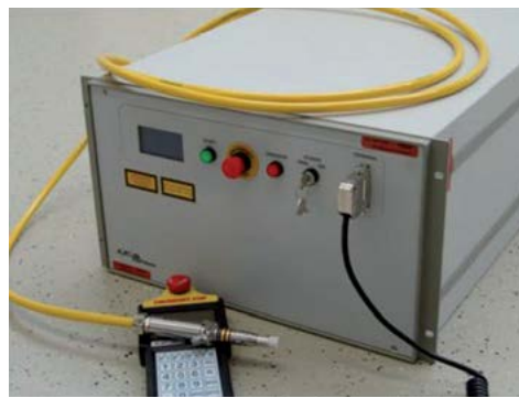
Fig. 4. Single-mode fibre laser of a power restricted within a 400-1000 W range. Main applications of this machine include precise and highly precise cutting as well as spot and continuous welding
