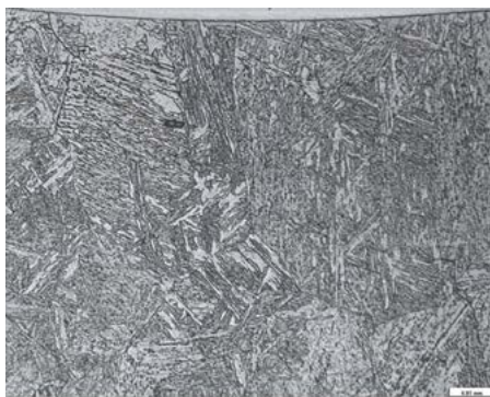
Fig. 8. Microstructure of the Heat Affected Zone of 10CrMo9-10 steel subjected to plasma surfacing using Inconel 625 alloy and the following process parameters: current of 100 A, surfacing rate of 20 cm/min and powder mass feeding rate 5 g/min, preheating to 200° etchant: Nital, mag. 500 x
