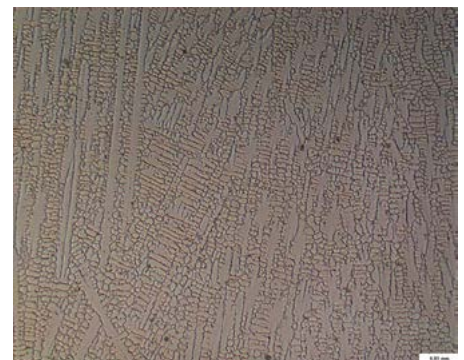
Fig. 13. Microstructure of the overlay weld made on 10CrMo9-10 steel using plasma surfacing and Inconel 625 alloy as well as the following process parameters: current of 150 A, surfacing rate of 30 cm/min and powder mass feeding rate 10.64 g/min, electrolytic etching, mag. 200 x
