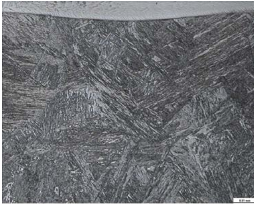
Fig. 7. Microstructure of the Heat Affected Zone of 10CrMo9-10 steel subjected to plasma surfacing using Inconel 625 alloy and the following process parameters: current of 100 A, surfacing rate of 20 cm/min and powder mass feeding rate 5 g/min, etchant: Nital, mag. 500 x
