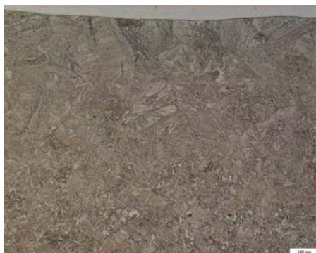
Fig. 11. Microstructure of the Heat Affected Zone of 10CrMo9-10 steel subjected to plasma surfacing using Inconel 625 alloy and the following process parameters: current of 150 A, surfacing rate of 30 cm/min and powder mass feeding rate 10.64 g/min, etchant: Nital, mag. 200 x
