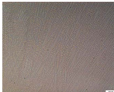
Fig. 12. Microstructure of the overlay weld made on 10CrMo9-10 steel using plasma surfacing and Inconel 625 alloy as well as the following process parameters: current of 90 A, surfacing rate of 30 cm/min and powder mass feeding rate 10.64 g/min, electrolytic etching, mag. 200 x
