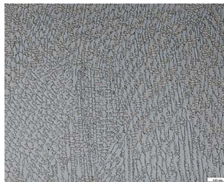
Fig. 9. Microstructure of the overlay weld made on 10CrMo9-10 steel using plasma surfacing and Inconel 625 alloy as well as the following process parameters: current of 100 A, surfacing rate of 20 cm/min and powder mass feeding rate 5 g/min, electrolytic etching, mag. 200 x
