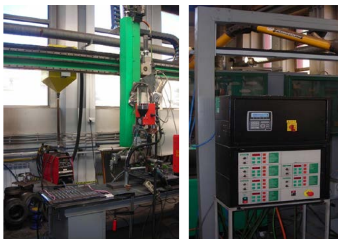
Fig. 2. Automated MultiSurfacer D2 Weld gantry for surfacing along with a control system, powder feeder and plasma torch
