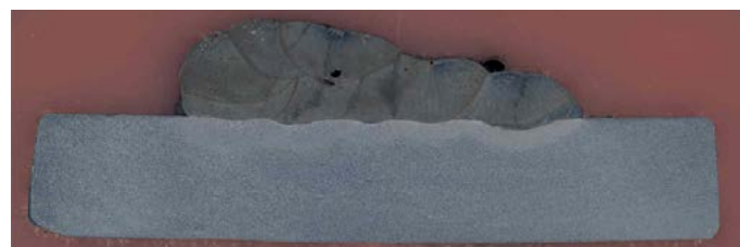
Fig. 13. Macrostructure of the overlay weld made using a Castolin EC 4119 covered electrode, (visible overlay weld metal porosity), etching: Adler's reagent
