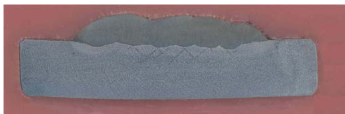
Fig. 12. Macrostructure of the overlay weld made using a Castolin EC 3292 covered electrode, etching: Adler's reagent
