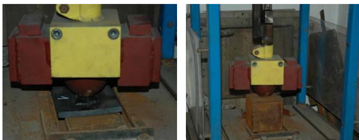
Fig. 6. Device for testing the resistance of overlay welds to impact loads
