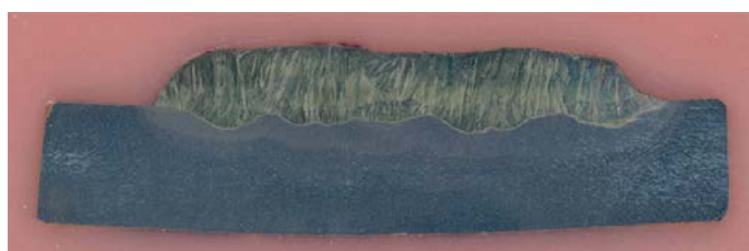
Fig. 10. Macrostructure of the overlay weld made using an ESAB EN 400MnB covered electrode, etching: Adler's reagent
