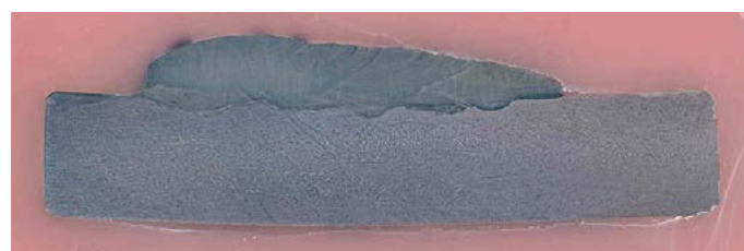
Fig. 11. Macrostructure of the overlay weld made using an ESAB EN 600B covered electrode, etching: Adler's reagent
