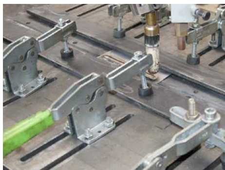
Fig. 1. Tooling used in the technological tests of the braze welding process
