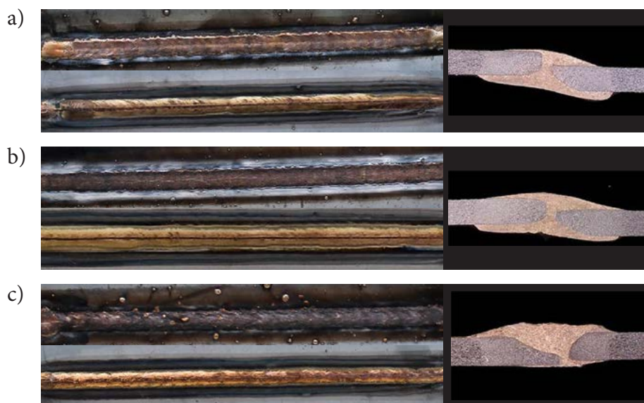
Fig. 5. Face (top), the other side of the specimen and the macrostructure of the butt joints made using the flux-cored wire and argon (a), Ar+1% O 2 mixture (b) and Ar+18% CO 2 mixture (c)
