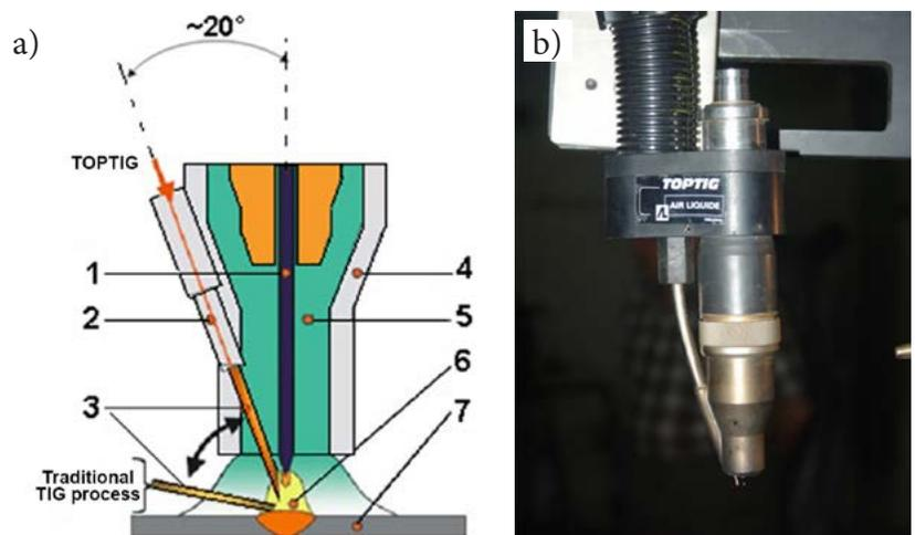
Fig. 1. (a) - Standard TIG welding torch with side wire feeding and TOPTIG welding torch: 1: tungsten electrode, 2: wire feeding conduit, 3: electrode wire, 4: gas nozzle, 5: shielding gas, 6: electric arc, 7: element being welded; (b) - TOPTIG welding torch
