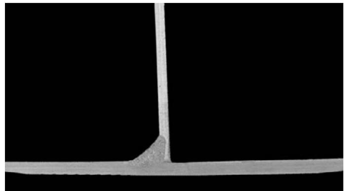
Fig. 9. Macrostructure of the T-joint made using the parameters presented in Table 5
