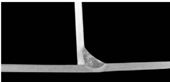
Fig. 5. Macrostructure of the T-joint made of 1.5 mm thick sheets using the parameters presented in Table 3
