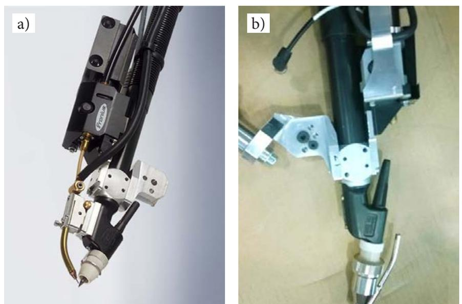
Fig. 8. Machine welding torch Robacta TTW4500: a) with the classical, i.e. side wire feeding [7]; b) after replacing the typical wire feeding unit with the unit incorporating a nozzle with a TOPTIG type wire feeding conduit
