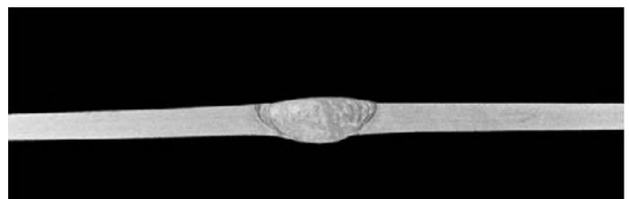
Fig. 4. Macrostructure of the T-joint made of 1.5 mm thick sheets using the TOPTIG method and the parameters presented in Table 2
