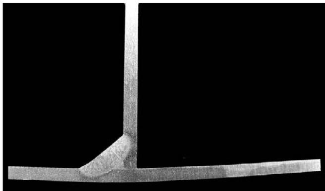
Fig. 7. Macrostructure of the T-joint made of sheets using the LORCH V 40 AC/DC welding machine and the parameters presented in Table 4
