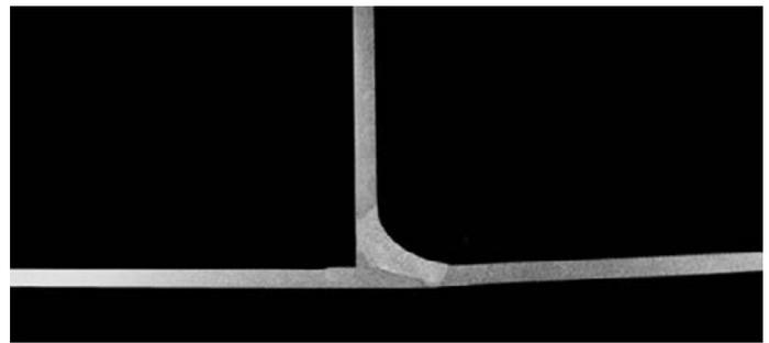
Fig. 3. Macrostructure of the T-joint made of 1.5 mm thick sheets using the TOPTIG method and the parameters presented in Table 1
