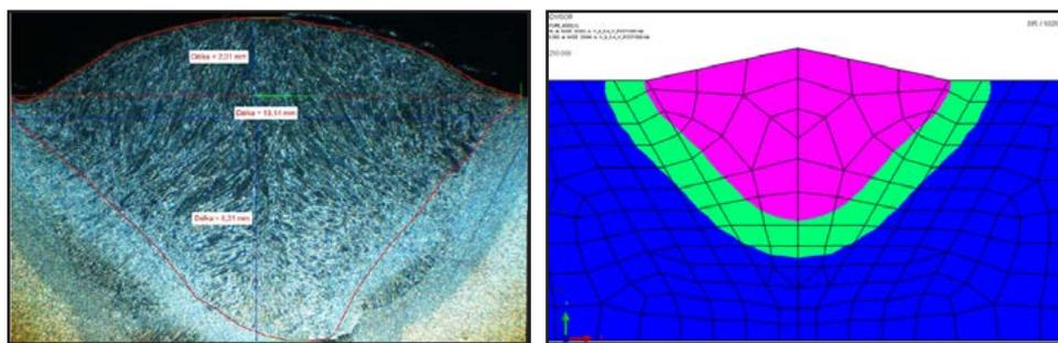
Fig. 5. Macrostructure of the butt joint bead made of S355 steel, the shape of the liquid metal pool corresponding to the macrostructure and the HAZ area during a numerical simulation
