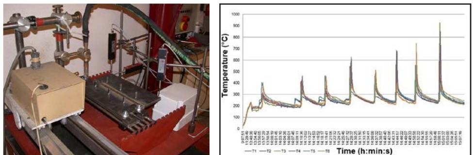
Fig. 3. Welding station used in tests and exemplary thermal cycles recorded when welding joints made of S355 steel
