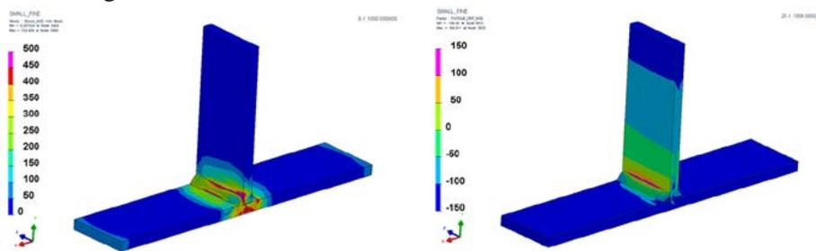
Fig. 2. Distribution of post-weld stresses and the result of high-cycle load analysis according to the Van Dang criterion
