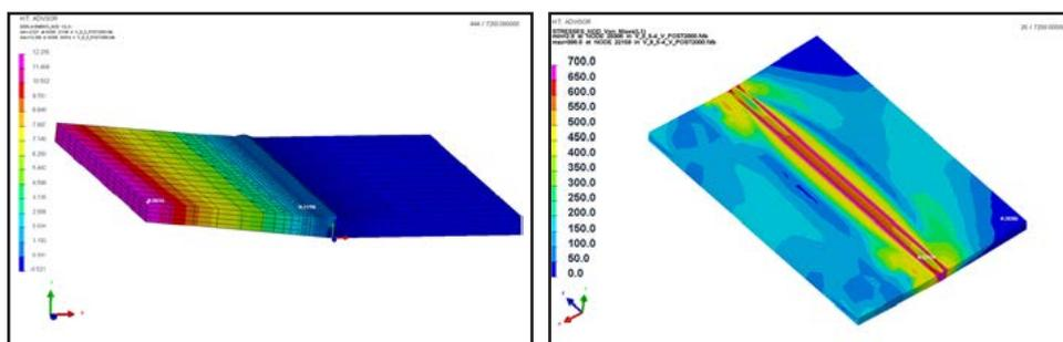
Fig. 6. Distribution of post-weld joint strains (left) and stresses (right)
