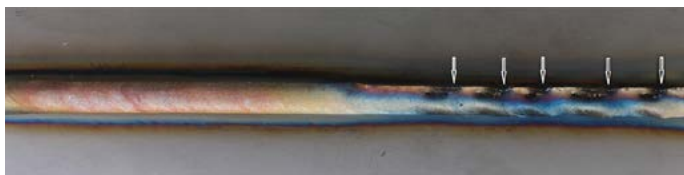
Fig. 2. View of the weld face after the change of a stable process (regular weld face surface) into unstable, caused by filler metal wire feeding disturbances (areas of disturbances are marked with arrows)
