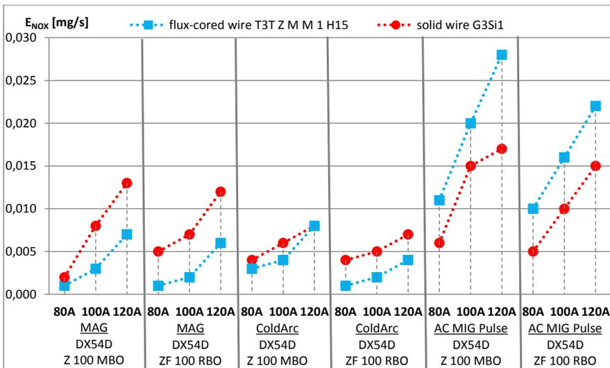
Fig. 6. Emission of nitrogen oxides during the 82%Ar+18%CO<sub>2</sub>-shielded MAG, ColdArc and AC MIG Pulse welding of protectively coated sheets involving the use of solid wire grade G3Si1 and flux-cored wire grade T3T Z M M 1 H15
