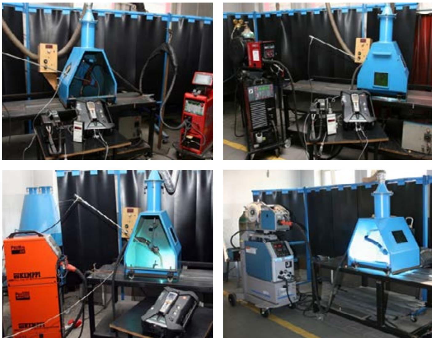
Fig. 1. Test rig for investigating the emission of welding fumes during the CMT, ColdArc, MAG and AC MIG Pulse welding process
