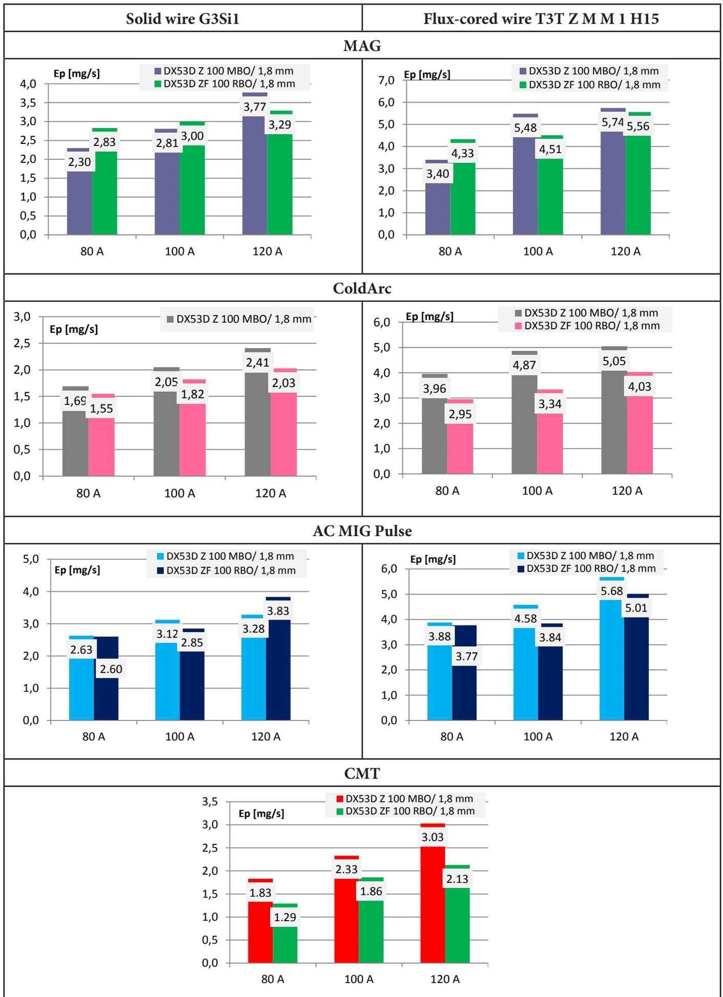
Fig. 4. Effect of the protective coating type of the steel sheets on the emission of total dust during MAG, ColdArc and AC MIG Pulse welding shielded by gas mixture 82% Ar + 18% CO<sub>2</sub>
