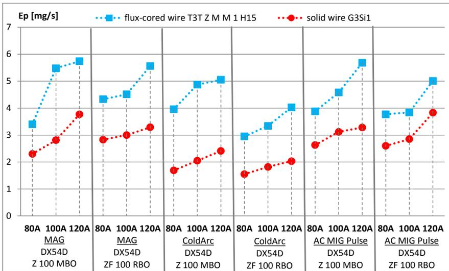
Fig. 5. Emission of total dust during the 82%Ar+18%CO<sub>2</sub>-shielded MAG, ColdArc and AC MIG Pulse welding of protectively coated sheets involving the use of solid wire grade G3Si1 and flux-cored wire grade T3T Z M M 1 H15
