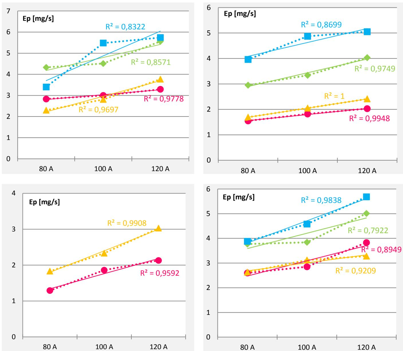
Fig. 8. Correlation between current and the emission of dust in relation to the MAG, ColdArc, AC MIG Pulse and CMT welding of protectively coated sheets performed using the solid wire and the flux-cored wire
