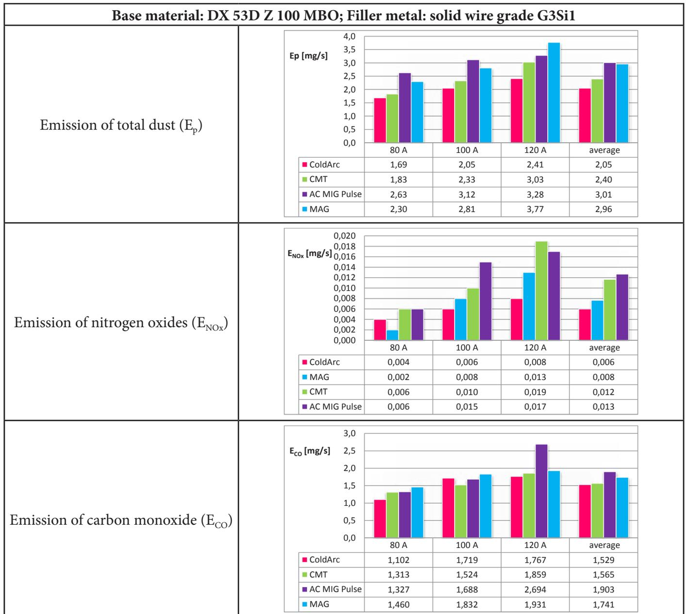
Fig. 2. Emission of welding fume during the 82%Ar+18% CO<sub>2</sub>-shielded welding of plate DX54D Z 100 MBO using solid wire grade G3Si1
