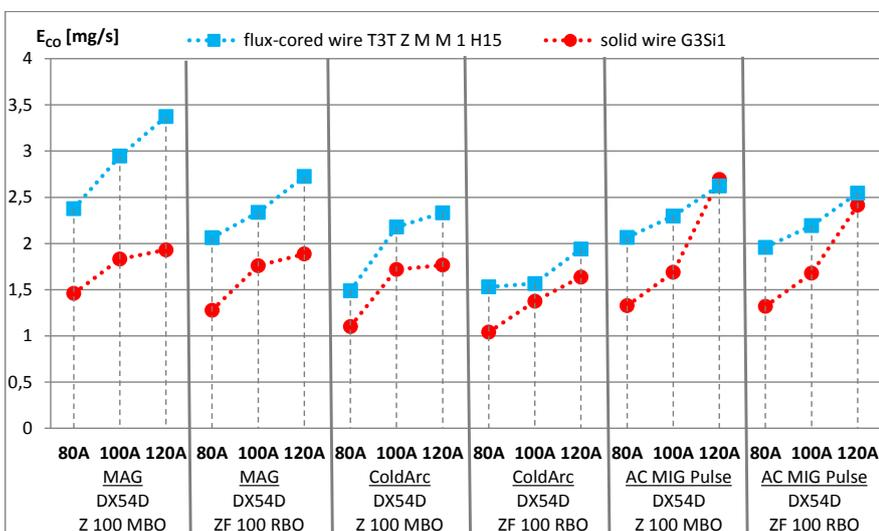
Fig. 7. Emission of carbon monoxide during the 82%Ar+18%CO<sub>2</sub>-shielded MAG, ColdArc and AC MIG Pulse welding of protectively coated sheets involving the use of solid wire grade G3Si1 and flux-cored wire grade T3T Z M M 1 H15
