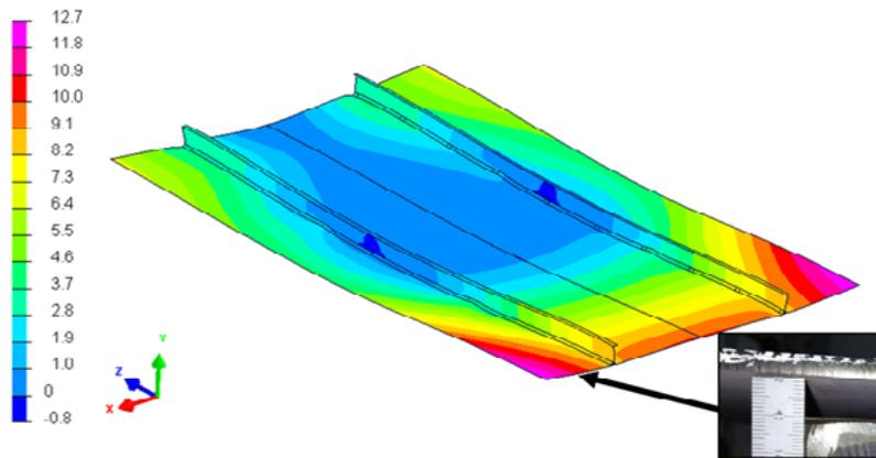
Fig. 13. Field of displacements in the normal direction in relation to the section subjected to welding in variant “0”, mm
