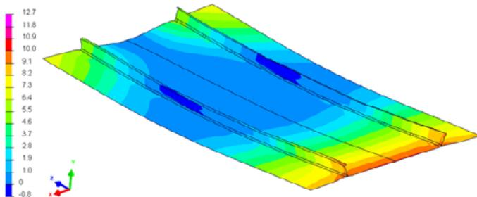
Fig. 18. Field of displacements in the normal direction in relation to the surface of the section welded in variant "2", mm
