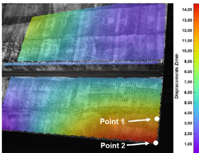
Fig. 10. Fragment the element subjected to welding with the superimposed field of displacement in the direction perpendicular to the surface of the flat section after the completion of the welding process, point 1 – maximum displacement (14.1 mm)
