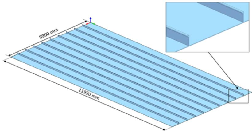
Fig. 4. Geometry of the flat sections and the bracing of group I
