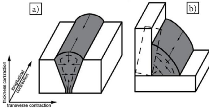
Fig. 1. Directions of volume changes in a) butt welds and b) fillet welds during post-weld cooling
