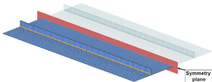
Fig. 11. Discrete model of the flat section and first-order bracings used in calculations and the plane according to which the boundary symmetry condition was preset
