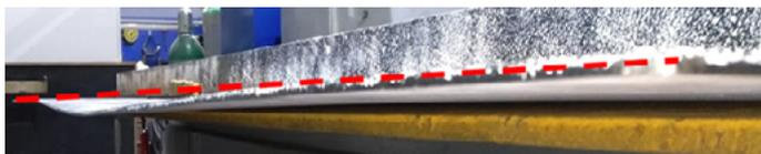
Fig. 9. Corrugated edge of the flat section after the completion of the welding process
