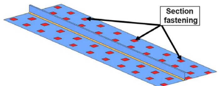
Fig. 16. Variant “2” of the fastening – section “fastened” to the welding table in selected areas (areas marked red)
