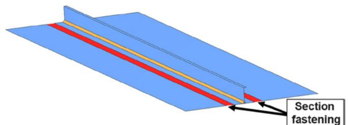
Fig. 15. Variant “1” of the fastening – section pressed against the welding table along the weld (areas marked red)
