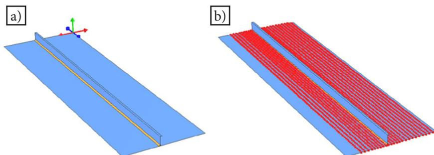
Fig. 12. Preset boundary conditions a) all-directional fastening and b) “stop” boundary condition
