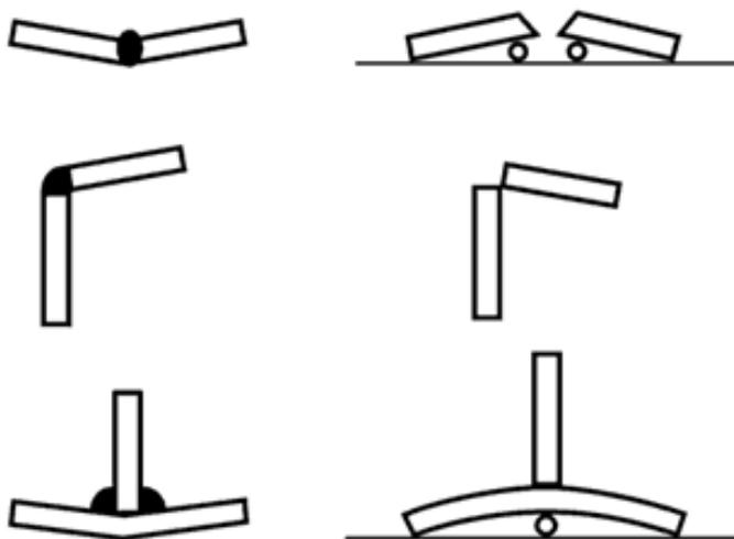
Fig. 2. Prevention of deformations: deformation is presented on the left, whereas the pre-weld deformation preventing the post-weld deformation is presented on the right [8]
