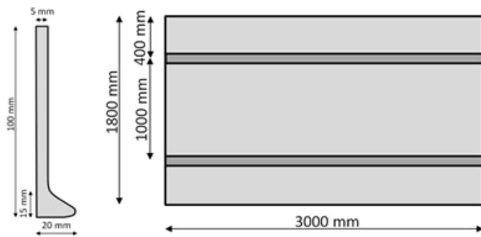
Fig. 6. Dimensions of the flat section and the arrangement of the first-order bracings
