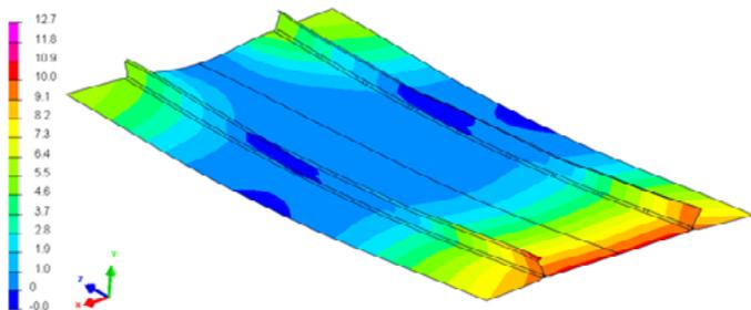
Fig. 17. Field of displacements in the normal direction in relation to the surface of the section welded in variant "1", mm
