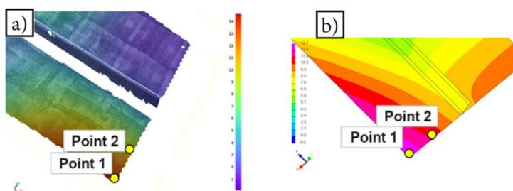
Fig. 14. Displacement in the normal direction in relation to the surface of the section welded in variant “0”
