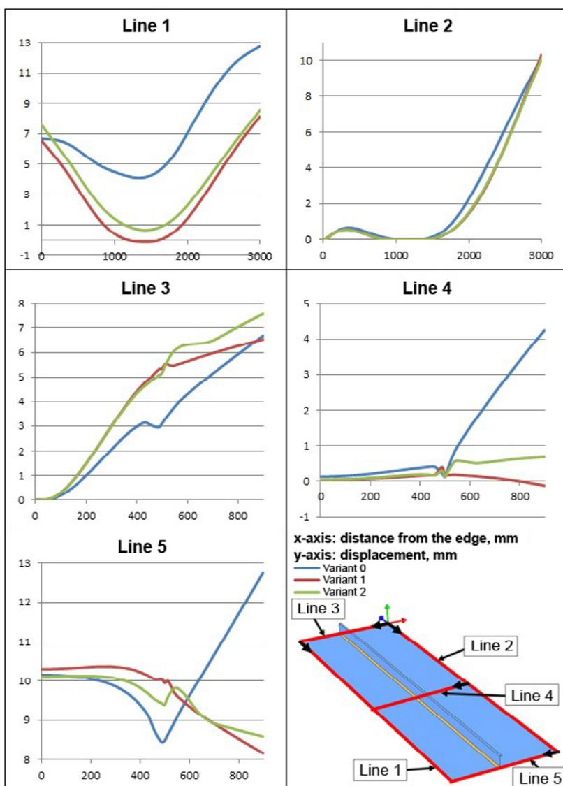
Fig. 19. Displacement of the nodes along selected lines in 3 analysed variants of element fastening during welding
