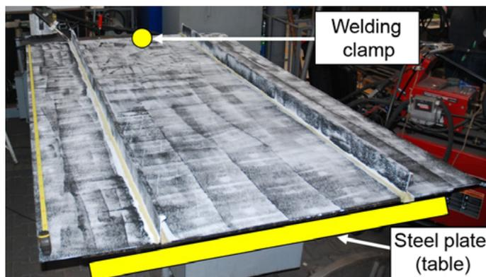
Fig. 7. Fastening flat section and first-order bracings during welding
