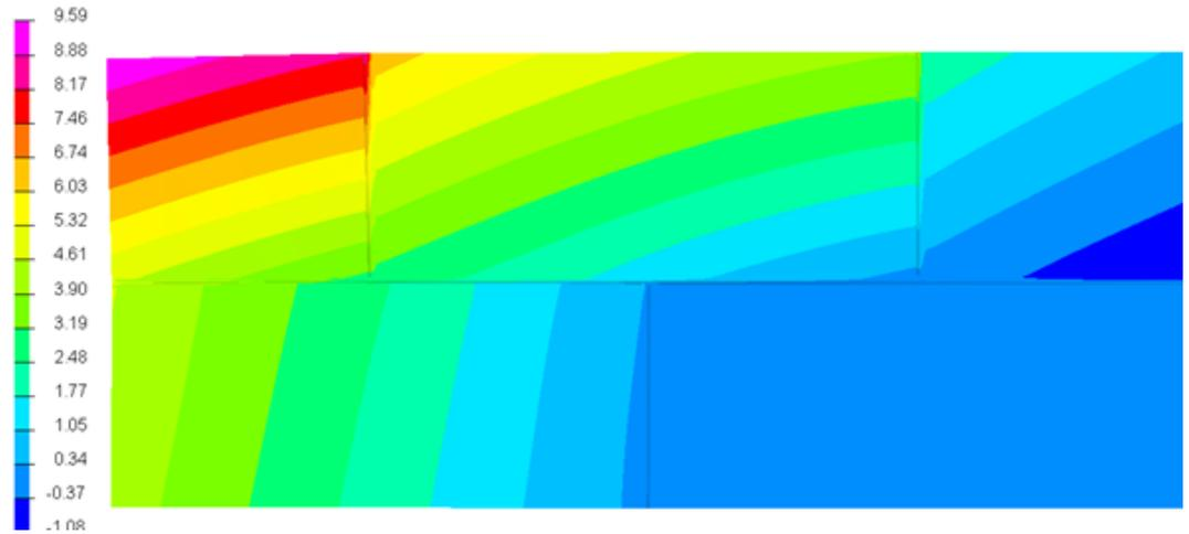
Fig. 5. Calculated field of displacement in the direction perpendicular to the surface of the element subjected to welding with the fastening of one sheet, mm [32]
