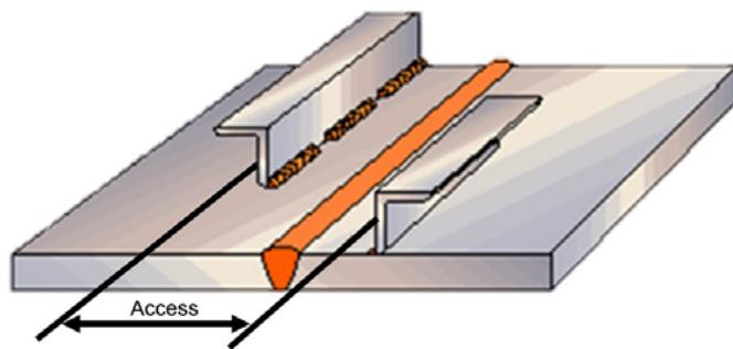
Fig. 3. Longitudinal stiffening preventing the deformation of thin butt-welded joints [9]
