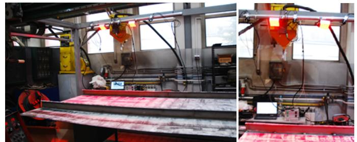
Fig. 8. Fragment of the flat section and bracings prepared for the measurements of welding distortions and the Dantec Dynamics Q-400 Multicamera Digital Image Correlation system
