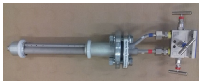
Fig. 5. Probe (Twin Bar) along with the flange and the system of valves
