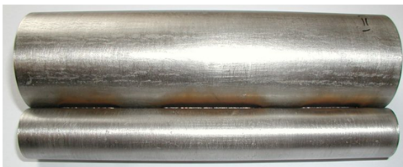
Fig. 2. Joining of the pipes welded at 20 mm long segments
