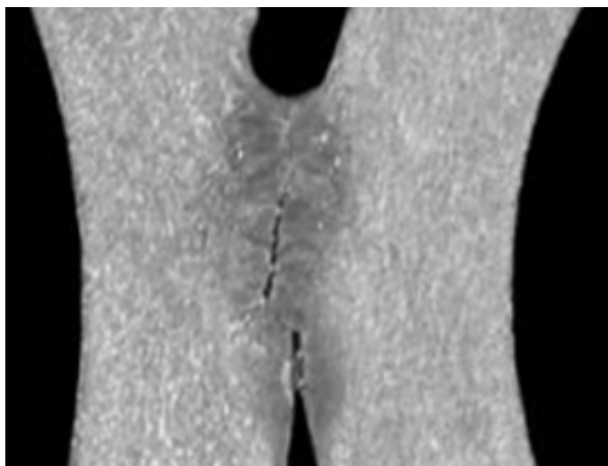
Fig. 4. Macrostructure of the laser welds in the impact pressure tubes made of steel X10CrAlSi25: a) cracks in the root of the weld made using the focused laser beam and b) proper weld made using the defocused laser beam [11]
