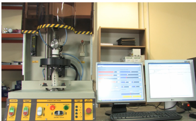
Station for the testing of structural transformations (developed and made at Instytut Spawalnictwa)
