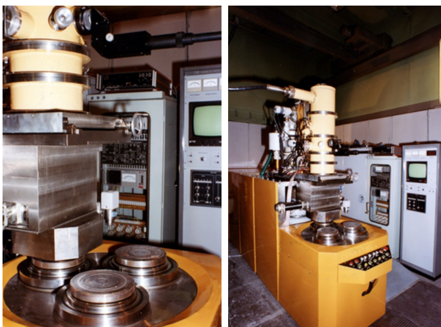
Electron beam welding SE 20-10/60 developed and made at Instytut Spawalnictwa
