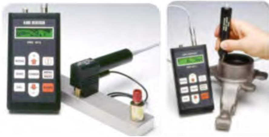
Fig. 5. Measurements performed using straight and angular potential transducers [4] sufficient accuracy. Figure 5 presents an exemplary measurement involving the use of a potential transducer.
