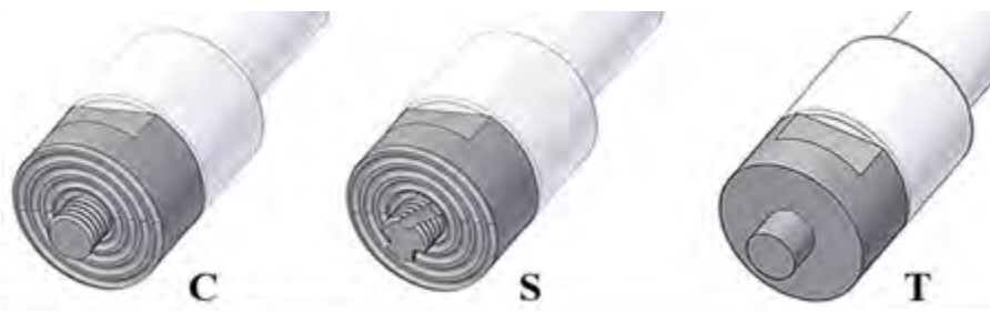
Fig. 2. Schematic view of FSW tools
