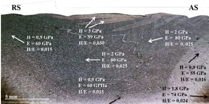
Fig. 10. The distribution of hardness (H), modulus of elasticity (E) and resistance to deformation (H/E) in the microstructure of T-type tool of FSW joint
