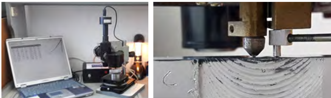
Fig. 4. The device "Micron-gamma" (a) in the process of recording the diagram of continuous indentation of the indenter into the material (b)
