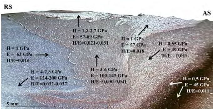
Fig. 8. The distribution of hardness (H), modulus of elasticity (E) and resistance to deformation (H/E) in the microstructure of C-type tool of FSW joint
