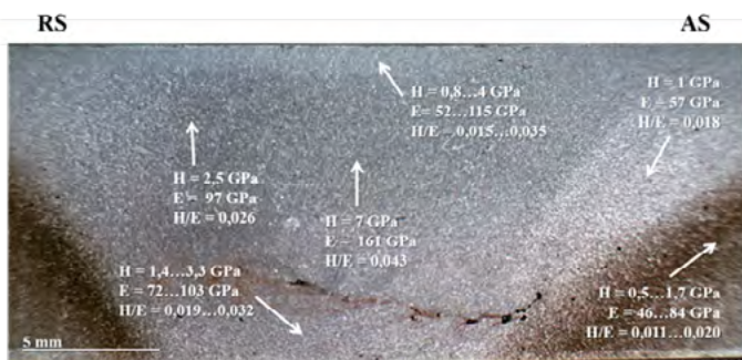
Fig. 9. The distribution of hardness (H), modulus of elasticity (E) and resistance to deformation (H/E) in the microstructure of S-type tool of FSW joint
