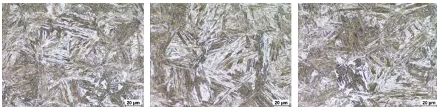
Fig. 3. Microstructure of steel S1300QL after simulation involving one thermal cycle in relation to cooling time  $t_{8/5} = 3$  s: a) heating 1x, martensite, hardness: 451 HV<sub>10av.</sub>, mag. 500x, b) heating 2x, martensite, hardness 466 HV<sub>10av.</sub>, mag. 500x, and c) heating 3x, martensite, hardness 462 HV<sub>10av.</sub>, mag. 500x
