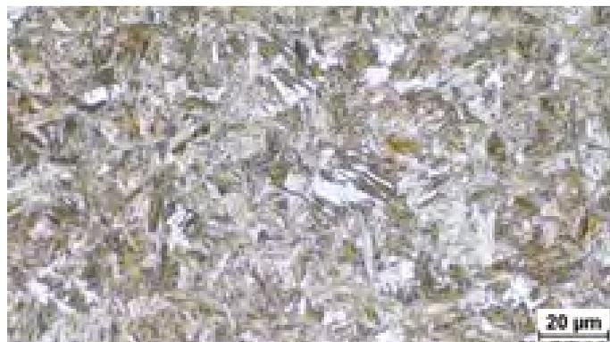
Fig. 2. Base material of steel S1300QL: martensite, hardness: 486 HV<sub>10av.</sub>, mag. 500x
