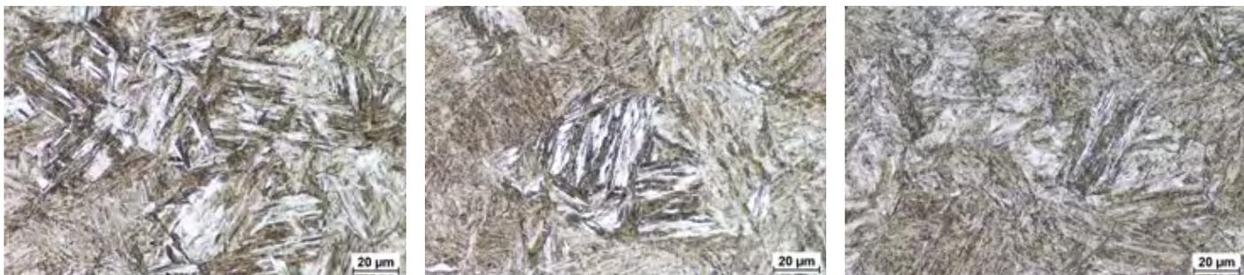
Fig. 5. Microstructure of steel S1300QL after simulation involving one thermal cycle in relation to cooling time  $t_{8/5} = 10$  s: a) heating 1x, martensite, hardness: 482 HV $_{10_{av}}$ , mag. 500x, b) heating 2x, martensite, hardness 486 HV $_{10_{av}}$ , mag. 500x, and c) heating 3x, martensite, hardness 433 HV $_{10_{av}}$ , mag. 500x
