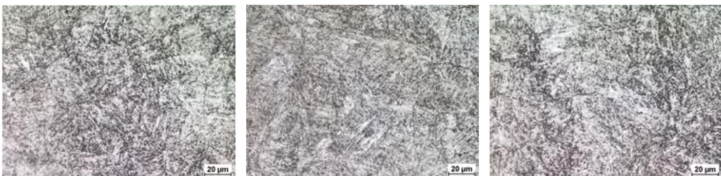
Fig. 6. Microstructure of steel S1300QL after simulation involving double thermal cycle ( $T_{max1} = 1250^{\circ}\text{C} + T_{max2} = 600^{\circ}\text{C}$ ) in relation to cooling time  $t_{8/5} = 5$  s: a) heating 1x, mixture of bainite and martensite, hardness: 344 HV $_{10_{av}}$ , mag. 500x, b) heating 2x, mixture of bainite and martensite, hardness: 339 HV $_{10_{av}}$ , mag. 500x and c) heating 3x, mixture of bainite and martensite, hardness: 339 HV $_{10_{av}}$ , mag. 500x
