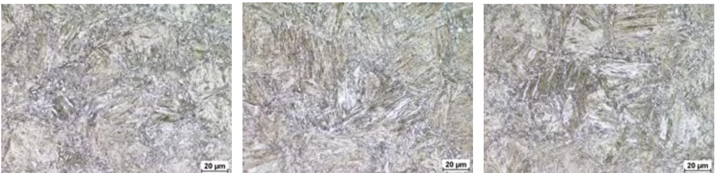
Fig. 11. Microstructure of steel S1300QL after simulation involving double thermal cycle ( $T_{max1} = 1250^{\circ}\text{C} + T_{max2} = 900^{\circ}\text{C}$ ) in relation to cooling time  $t_{8/5} = 10$  s: a) heating 1x, martensite and traces of ferrite, hardness: 482 HV $_{10_{av}}$ , mag. 500x, b) heating 2x, martensite and traces of ferrite, hardness: 462 HV $_{10_{av}}$ , mag. 500x and c) heating 3x, martensite and traces of ferrite, hardness: 476 HV $_{10_{av}}$ , mag. 500x
