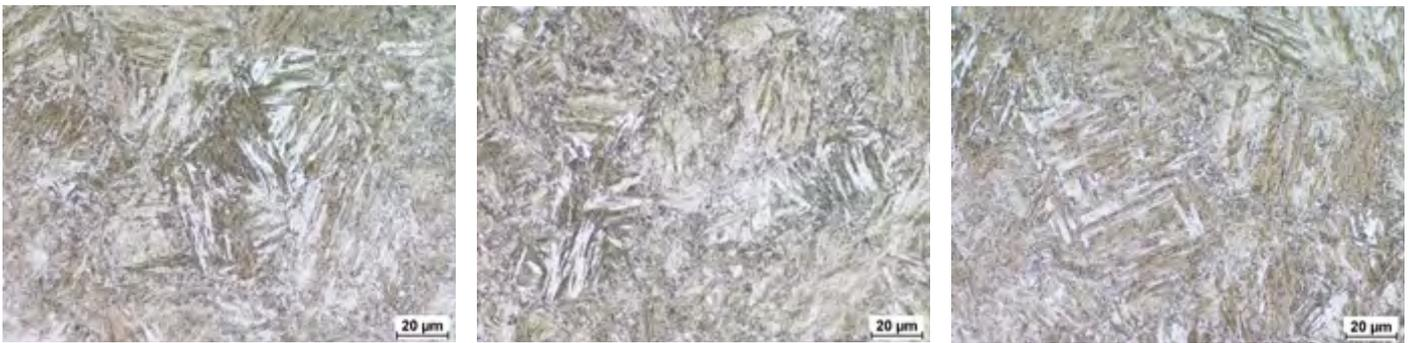
Fig. 10. Microstructure of steel S1300QL after simulation involving double thermal cycle ( $T_{max1} = 1250^{\circ}\text{C} + T_{max2} = 900^{\circ}\text{C}$ ) in relation to cooling time  $t_{8/5} = 5$  s: a) heating 1x, martensite and small amounts of ferrite, hardness: 474 HV $_{10_{av}}$ , mag. 500x, b) heating 2x, martensite and traces of ferrite, hardness: 483 HV $_{10_{av}}$ , mag. 500x and c) heating 3x, martensite and traces of ferrite, hardness: 478 HV $_{10_{av}}$ , mag. 500x
