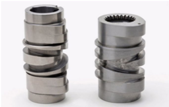
Fig. 5. Set of cams hardened using the electron beam; surface hardness >650 HV, hardness depth >0.4 mm [21]
