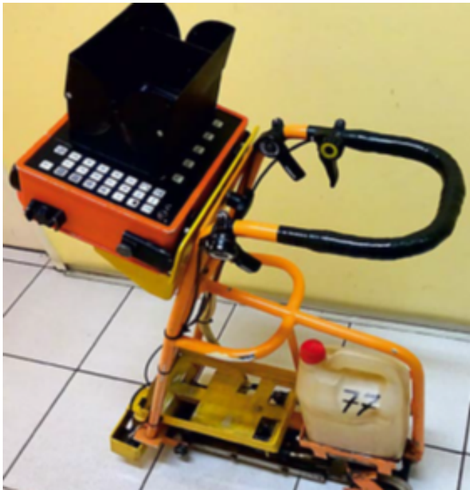
Fig 9. Track gauge (model RDM-12) [8]
