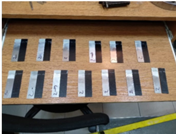
Fig. 7. Adhesive nature of the failure of the adhesive-bonded joints – the lack of visible adhesive “particles” on the surface of the composite material
