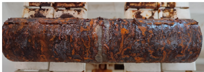
Fig. 17. Specimen after 168 hours' exposure in the salt spray chamber
