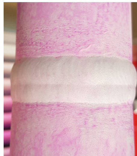
Fig. 13. Specimen with the developer applied
