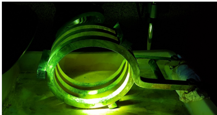
Fig. 14. Magnetic particle test rig – rigid coil
