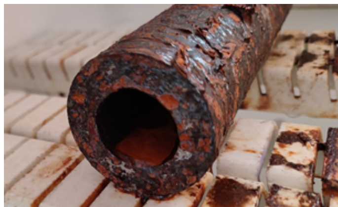
Fig. 18. Face of the specimen after 168 hours' exposure in the salt spray chamber
