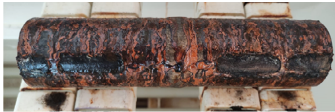
Fig. 16. Specimen after 48 hours' exposure in the salt spray chamber
