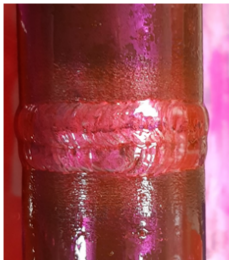
Fig. 12. Specimen with the penetrant applied
