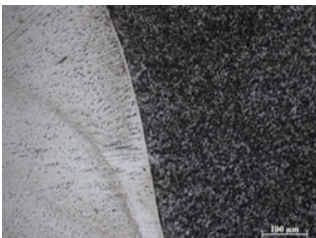
Fig. 7. Weld with the fusion line; mag. 200x
