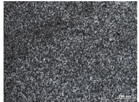
Fig. 6. Heat affected zone, normalisation area; mag. 200x
