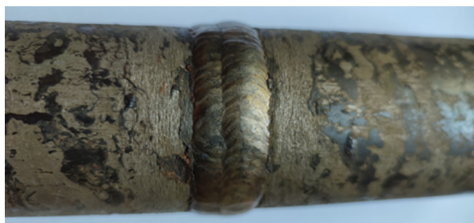
Fig. 19. Specimen of the corrosion resistance test with the corrosion products removed
