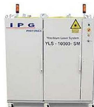
Fig. 4b. IPG-manufactured YLS-10000-SM fibre optic laser with a power of 10 kW [7]
