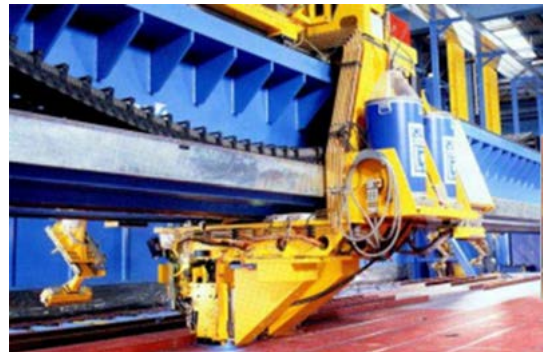
Fig. 8. Hybrid welding of ship deck plating panels, butt joints of plates and welding stiffening elements. Laser CO 2 , 12 kW. Shipyard Meyer, Germany [5]
