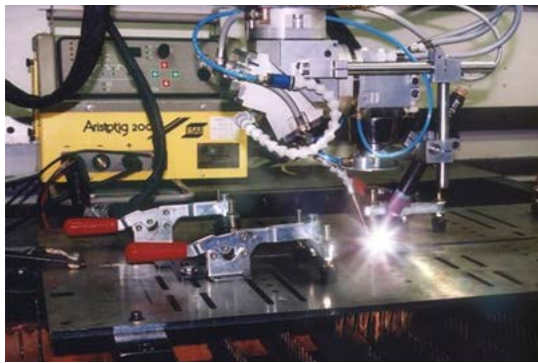
Fig. 7. Laboratory station for testing hybrid welding: Trumpf TLC 1005 CO 2 laser (3.8 kW); Esab-manufactured Aristotig 200 welding machine
