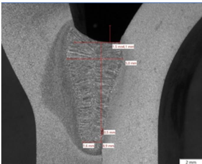
Fig. 4. Exemplary application of the laser beam in the making of a hard-to-access joint
