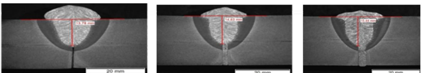
Fig. 1. Macrographic metallographic specimens of the cross-section of elements welded using high-current arc in relation to various sizes of the gap between the elements (square butt weld preparation)
