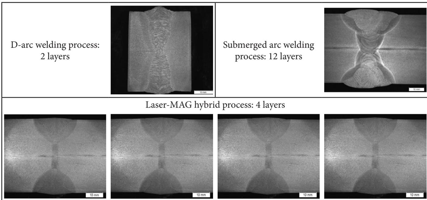
Fig. 9. Comparison of high-performance welding processes
