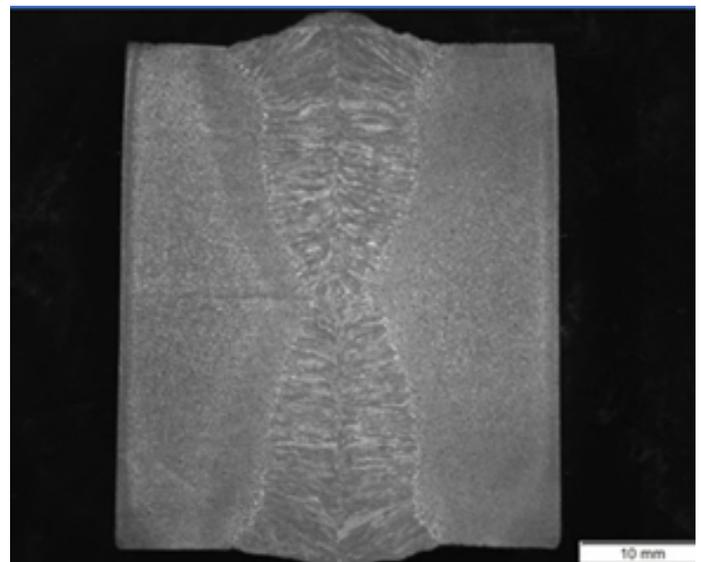
Fig. 2. Macrographic metallographic specimen of the cross-section of the elements subjected to two-sided arc welding process (with deep penetration)
