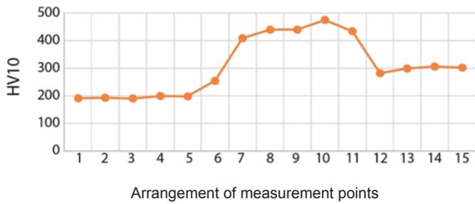
Fig. 6. Hardness distribution in the cross-section of the weld of the joint made of two different types of steel (Fig. 5)
