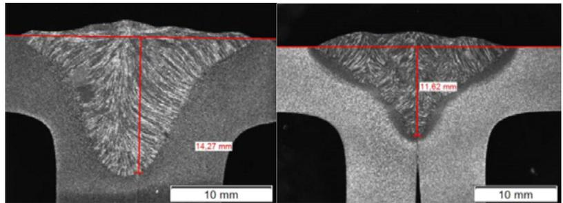
Fig. 3. Comparison of flare welds in accordance with ISO 2553; multi-run MAG weld (a); single-run D-arc weld
