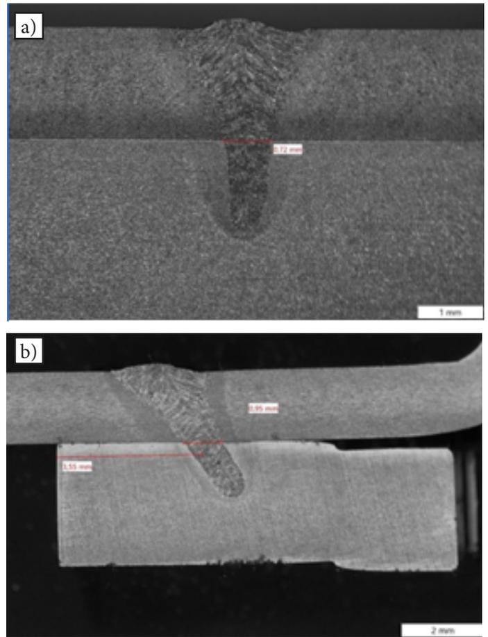
Fig. 7. Welds in the overlap joint made using the laser beam positioned at various angles: perpendicular position of the laser beam (a) and the laser beam positioned at an angle of 45° (b)
